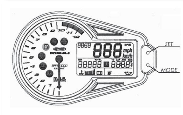
The dashboard contains two buttons in its right side, the upper one is to select “SET” and the lower one for the function “MODE.”
