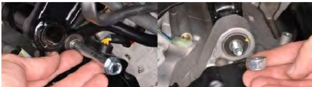
Insert the engine mounting bracket and damper bolt from the right side. Thread on the nut.
