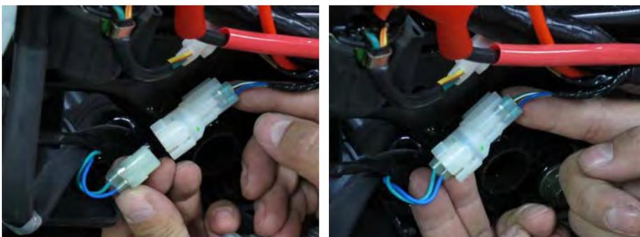
Plug in the crank position sensor wire coupler on the right side of the frame.
