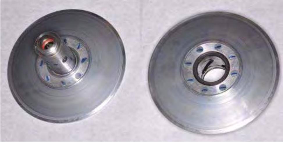
Inspect the faces of the driven pulley. Clean away any grease from the faces where the belt rides.
