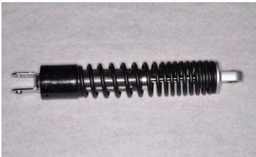
Fit the shock absorber into place. Make sure the preload arrow indicator faces out from the lower mount.
