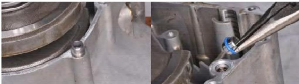
Remove the two dowel pins from the crankcase. Inspect the O-ring and replace it as needed.
