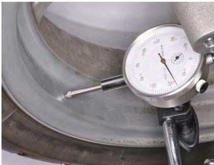
Check for radial hop. The service limit is 2.0 mm (0.08 in) or less.
