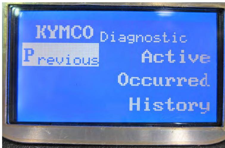
Pressing the enter button on the DTC Inspect item will bring up the options shown above.
