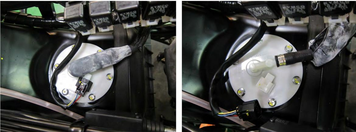
Inspect the fuel hose for signs of deterioration or damaged. Replace the fuel hose as needed.
