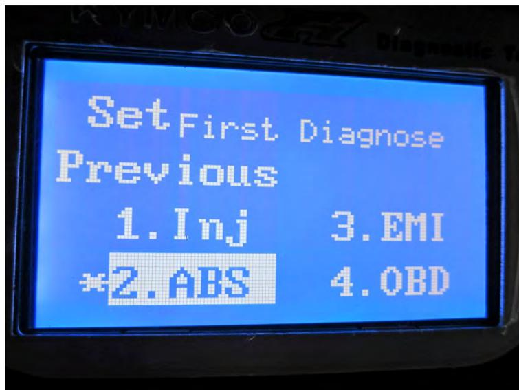
Connect the diagnostic tool and set the ECU to the ABS.
