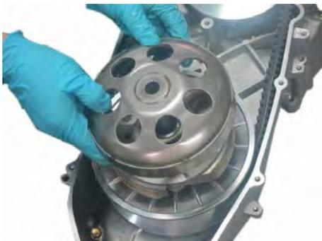
Remove the outer clutch.
