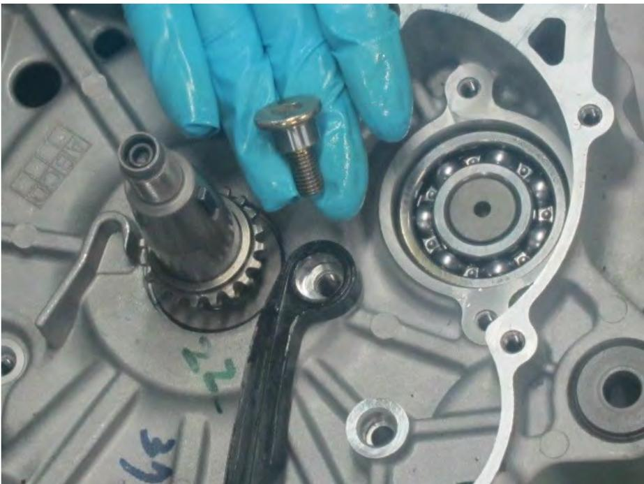
Remove the upper cam chain guide.
