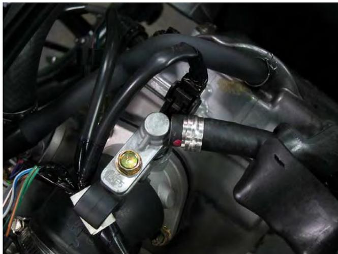
Slide back the clamp and free the injector fuel pipe from the fuel hose. Inspect the fuel hose for signs of deterioration or damaged. Replace the fuel hose as needed.
