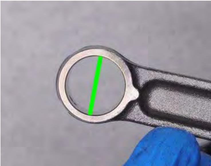
Measure the inside diameter of the small end of the connecting rod with vernier calipers.
