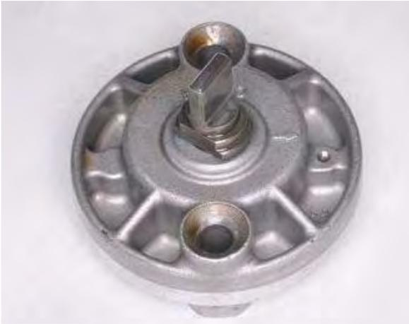
Turn the oil pump shaft by hand and make sure it turns smoothly. If the oil pump shaft will not rotate smoothly the oil pump should be replaced with a new unit.
