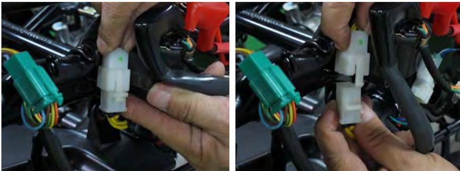
Plug in the regulator/rectifier 3-pin connector.
