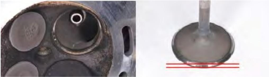
Inspect the valve seat and the valve seat width. The valve seat should be centered on the valve face. If the seat is pitted, worn out, or fits poorly on the valve face the valve seat must be resurfaced.
