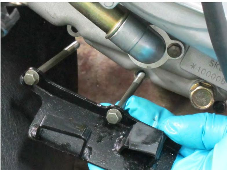
Remove the plate with the bottom two crankcase bolts.
