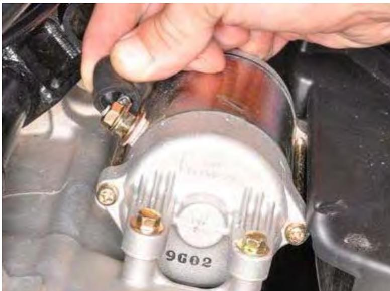
Fit the rubber starter motor lead cover into place.
