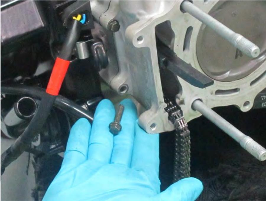
Thread in the two cylinder bolts on the right side of the engine.
