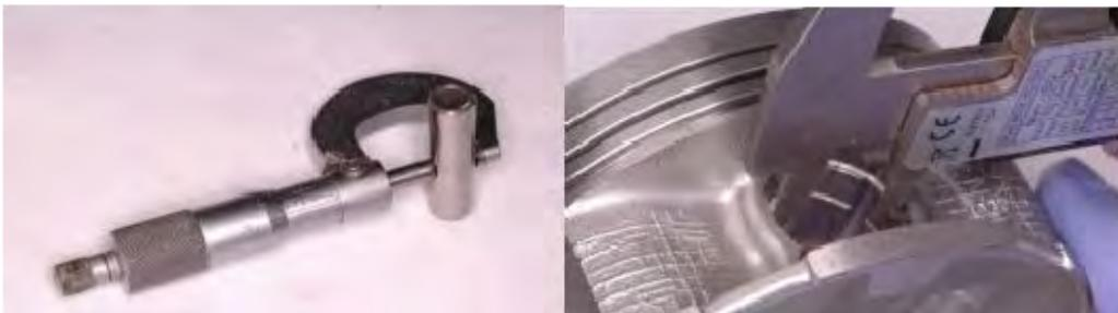
Measure the piston pin diameter with a micrometer. Measure the piston pin bore diameter with vernier calipers or a small bore gauge. Measuring at three different points for each. Replace the parts if any of the specifications are not met.
