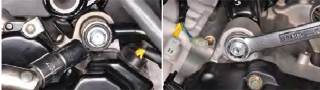
Tighten the engine mounting bracket damper bolt and nut with a 17 mm wrench for the nut and a 14 mm socket for the bolt.
