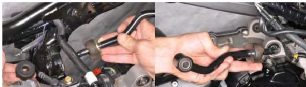
Remove the engine mounting bracket damper assembly.
