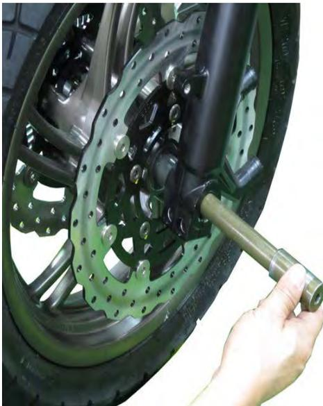
Apply a light coat of grease to the front axle. Insert the axle from the left side. Set the front wheel on the ground. Pump the front suspension up and down several times to seat the front axle.
