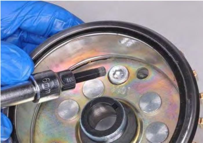
Tighten the starter clutch mounting bolts to specification with a 6 mm Allen socket.
