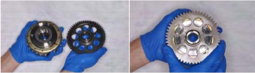
Fit the boss of the starter driven gear into the starter clutch. The starter clutch should only allow the driven gear to turn in one direction. If the starter clutch allows turning both ways or will not let the driven gear rotate smoothly in one direction the starter clutch must be replaced.
