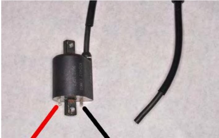
Touch the positive and negative meter leads to the ignition coil terminals as shown. Measure the resistance.
