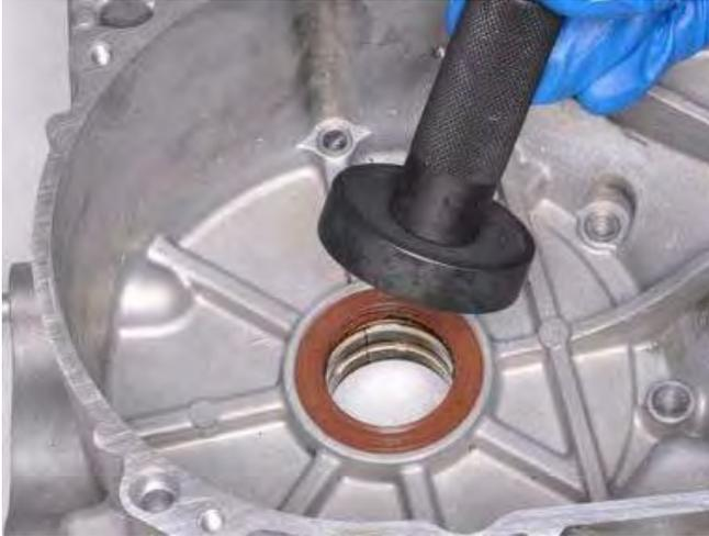
Drive the new seal into the left crankcase from the outside with a suitable driver. The driver should have the same outside diameter as the seal. Lubricate the new crankshaft seal lips with fresh engine oil.
