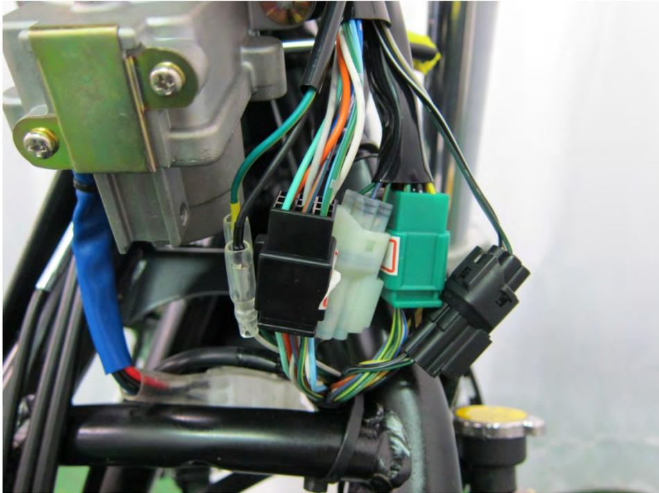
Unplug the black connector for the left handlebar switches.
