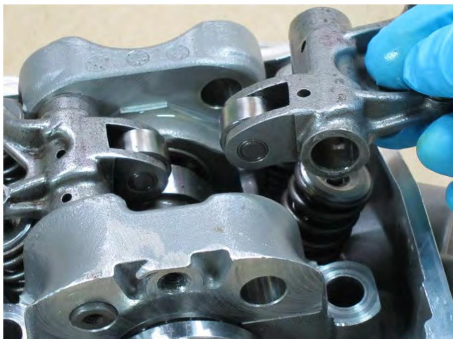
Lubricate the inside diameter of the rocker arms and the roller with fresh engine oil. Position the rocker arms to accept the rocker arm shafts.
