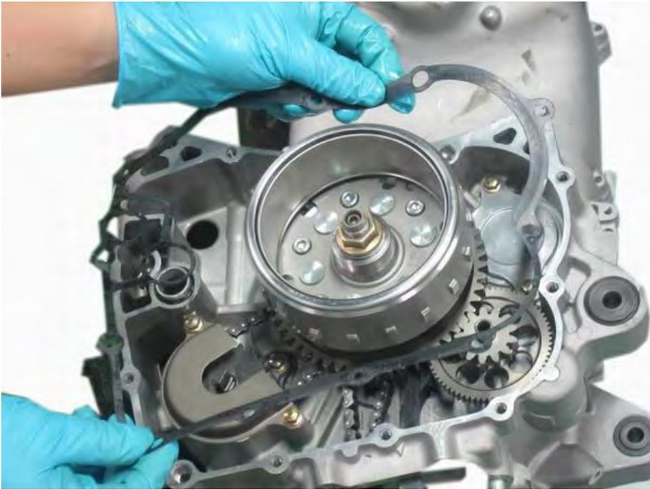
Remove the generator cover gasket.
