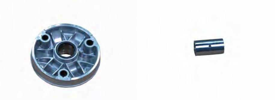
Inspect the movable drive face and bushing for wear and damage. Replace the parts as needed.
