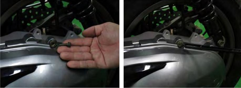
Insert the plastic cover bolts and tighten them securely with an 8 mm socket.
