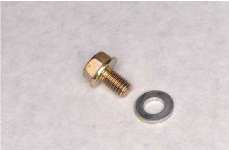
Inspect the drain plug and washer.
