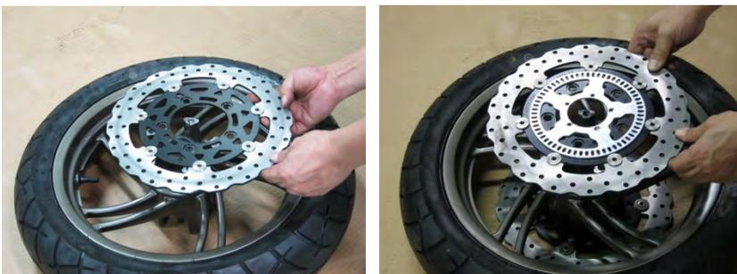
Remove the front brake discs.
