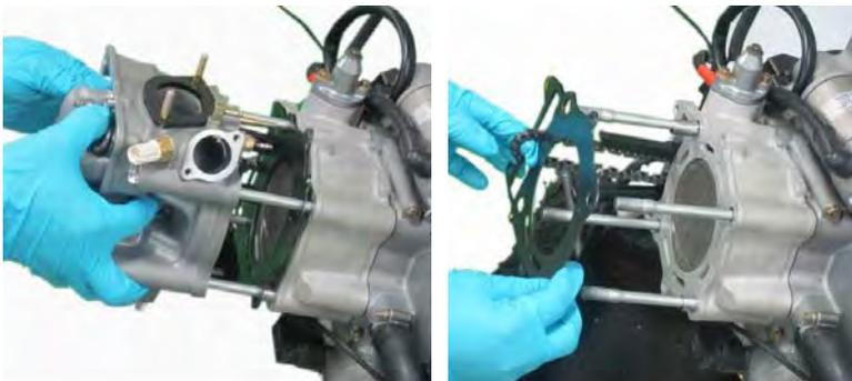
Remove the cylinder head assy and gasket.
