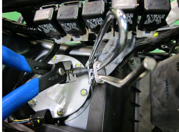
To separate the fuel hose from the fuel pump pipe.
