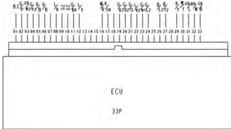
Check for continuity between pin 9 and 10 of the ECU side connector.
