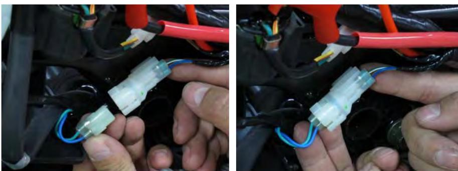
Disconnect the crank position sensor wire coupler.
