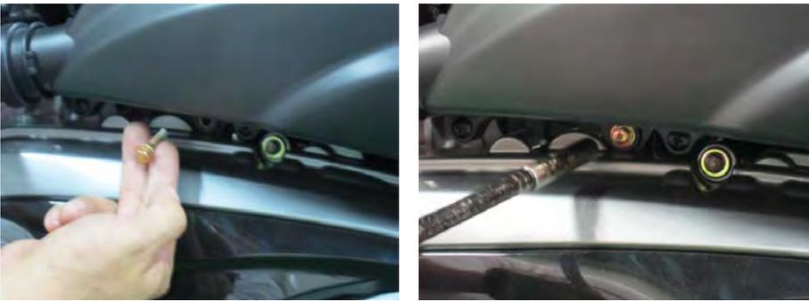
Install 2 the air cleaner bolts with an 8 mm socket.
