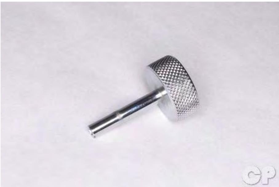
Use a tappet adjuster tool to adjust the valves.
