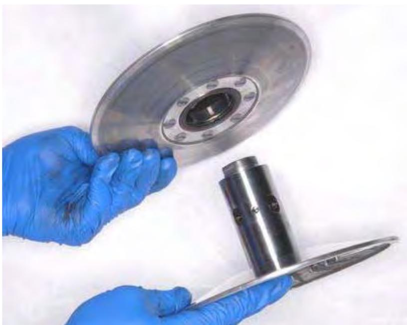
Separate the left and right faces of the driven pulley.
