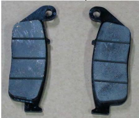
Replace the pads if the brake wear exceeds the wear indicator lines or if the wear is uneven.
