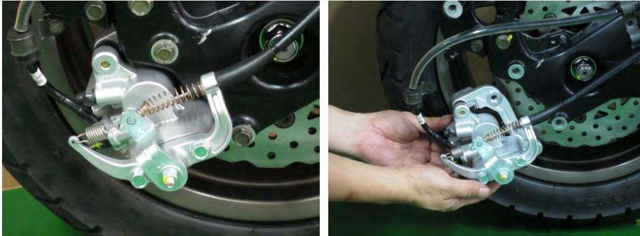
Place a suitable container under the banjo bolt to catch any remaining brake fluid. Remove the banjo bolt that holds the brake hose to the caliper using a 12 mm socket. Discard the two sealing washers.
