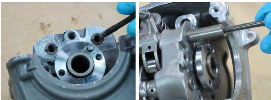
Thread a bolt into the rocker arm shafts and pull the shafts out.
