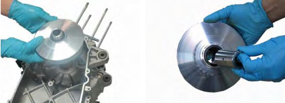
Remove the right (movable) face of the drive pulley from the crankshaft. Slide the bushing out of the movable drive face.
