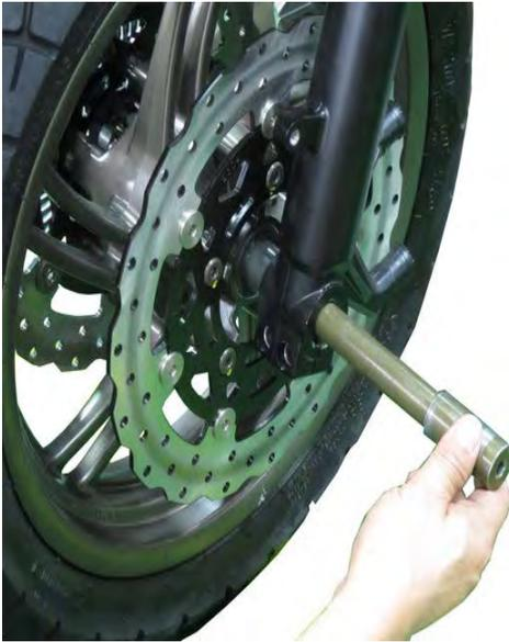
Support the front wheel and slide the front axle out from the left side.
