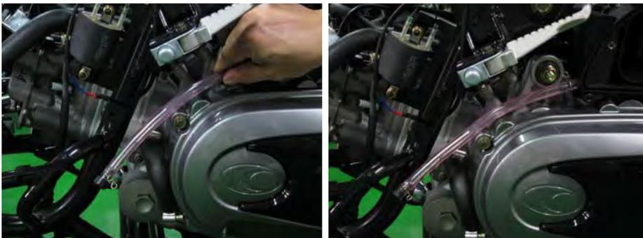
Fit the drain hose to the plastic belt case cover as shown.
