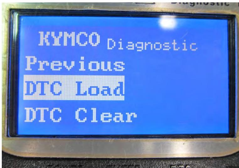
Press the down button to select the load DTC option. Press the enter button on the Load DTC item to display the DTC options.
