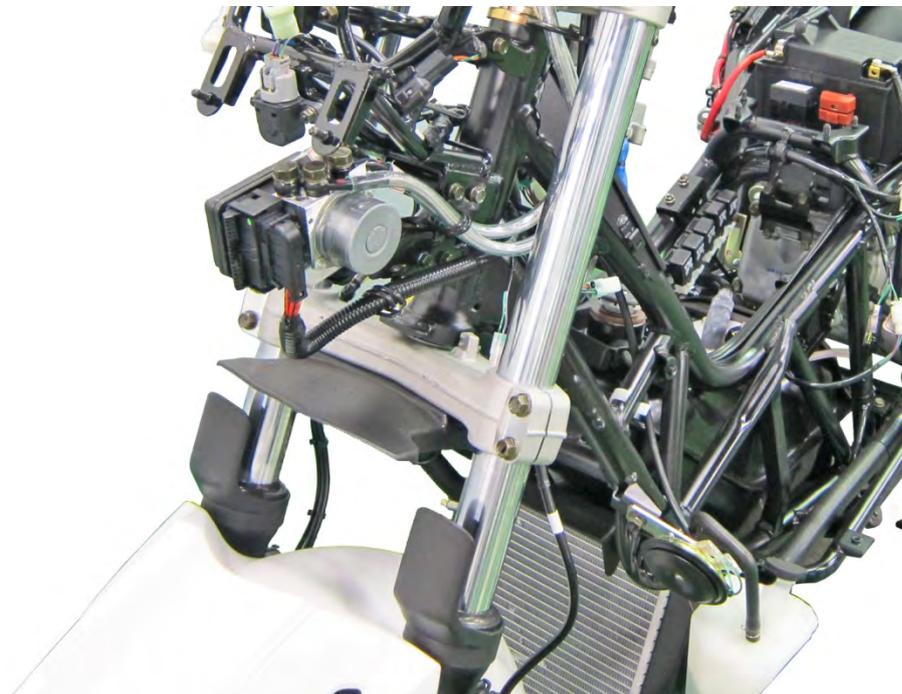
Loosen the coolant hose clamps with a #2 Phillips screwdriver.
