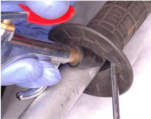
If you plan to replace the grips you can slice them lengthwise with a razor blade and peel them off. To remove the grips without cutting them use a screwdriver to open a gap between the grip and the handlebar. Spray in contact cleaner to break up the grip cement. Use compressed air to expand the grip so it can be easily slid off the end of the handlebar. Note the relationship between the angle of the grip and the throttle tube so that the new grip can be installed with the correct angle.
