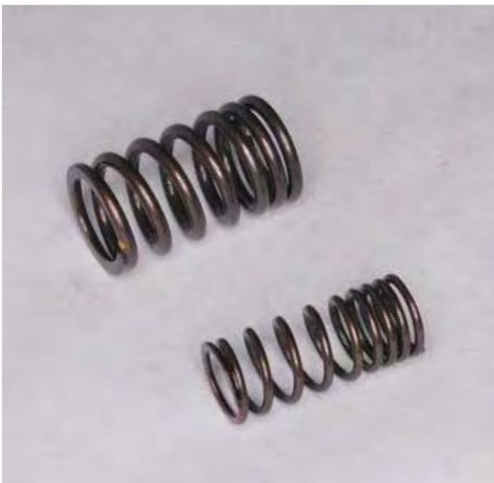
Inspect the valve springs for fatigue and damage. Replace the valve springs as needed or if the valve is also to be replaced.
