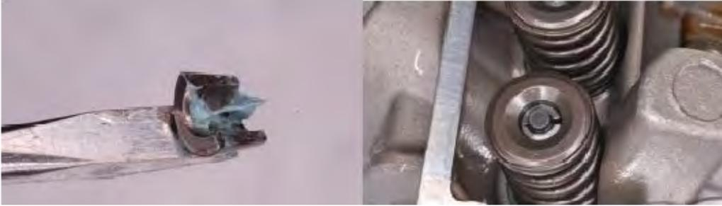
Apply grease to the inside of the split keepers. Apply a dab of grease to the end of a flat blade screwdriver. Set the keeper in the grease on the screwdriver and insert it onto the valve stem. Repeat this with the other keeper.
