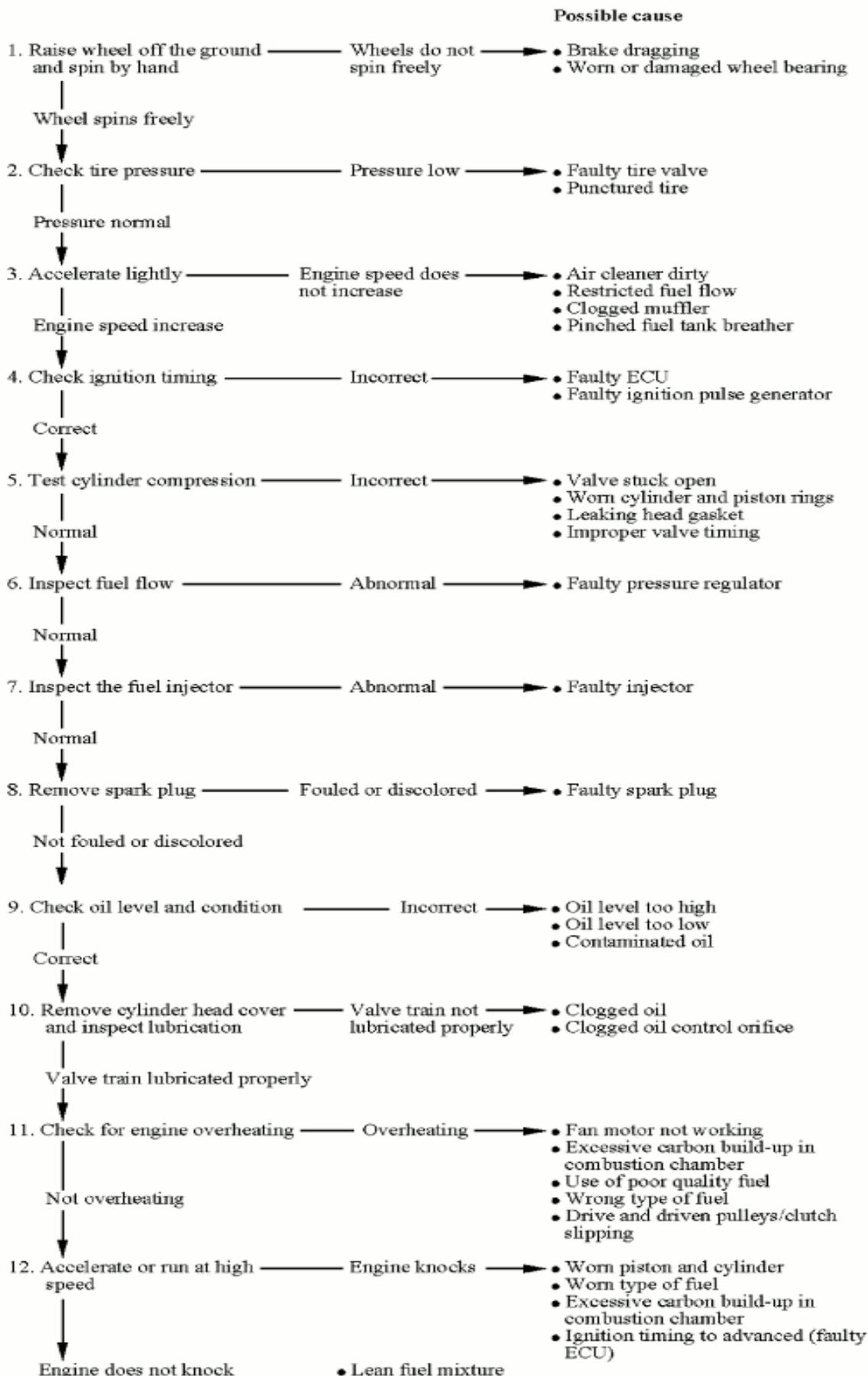
**POOR PERFORMANCE AT LOW AND IDLE SPEED**
