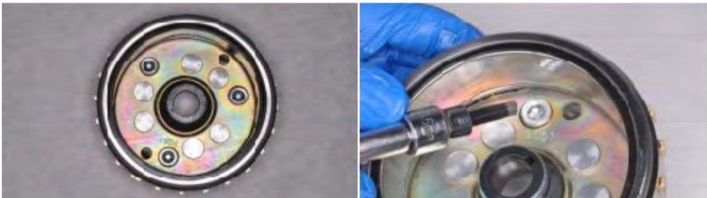
Remove the three starter clutch mounting bolts with a 6 mm Allen socket.
