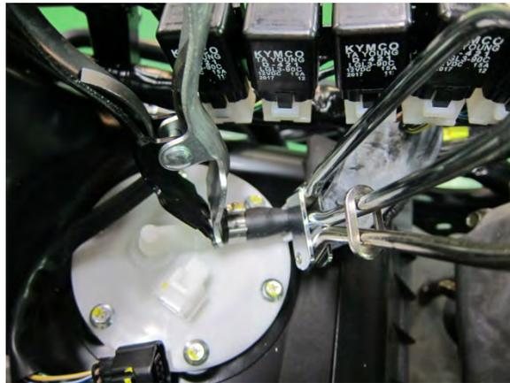
Remove the fuel pump mounting bolts. And remove the fuel pump assembly.
