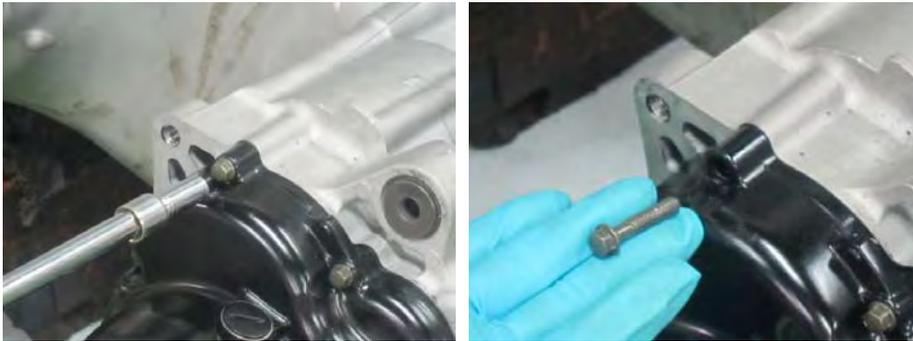
Remove the 12 generator cover bolts with an 8 mm socket.
