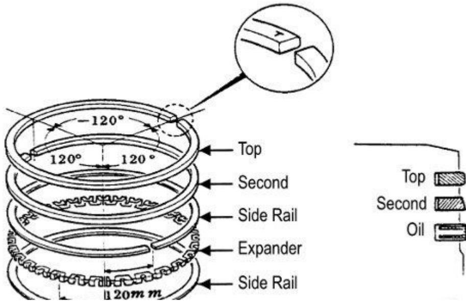
Install the top and second rings with their markings facing up. Install the rings to the piston as shown above so that no ring end gaps line up with the piston pin or perpendicular to the piston pin. The rings should turn easily on the piston without sticking or roughness.
