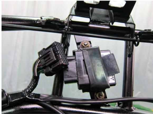
Remove the two nuts to remove the ECU.
