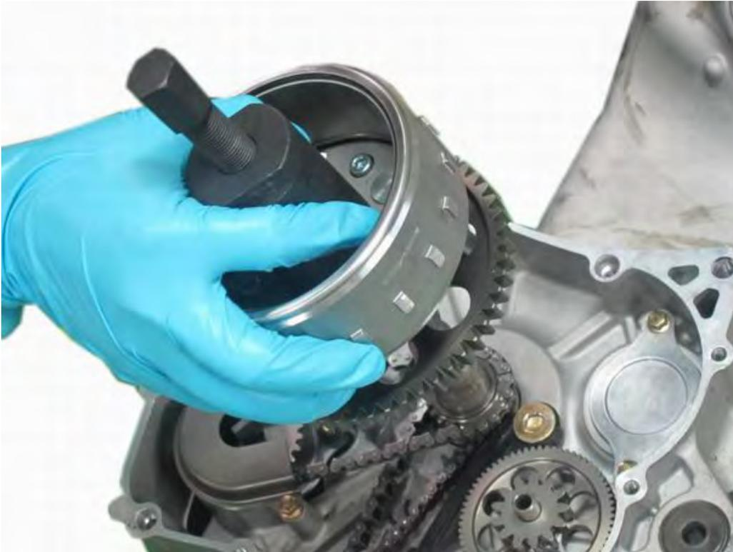
Remove the flywheel from the crankshaft.
