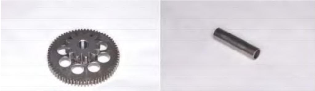
Inspect the starter idle gear and shaft for wear and damage. Replace the idle gear and shaft as needed.
