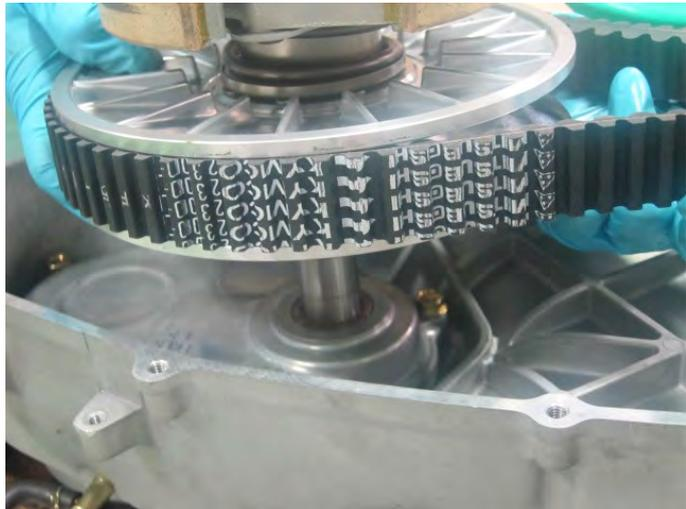
Remove the belt from the driven pulley.
