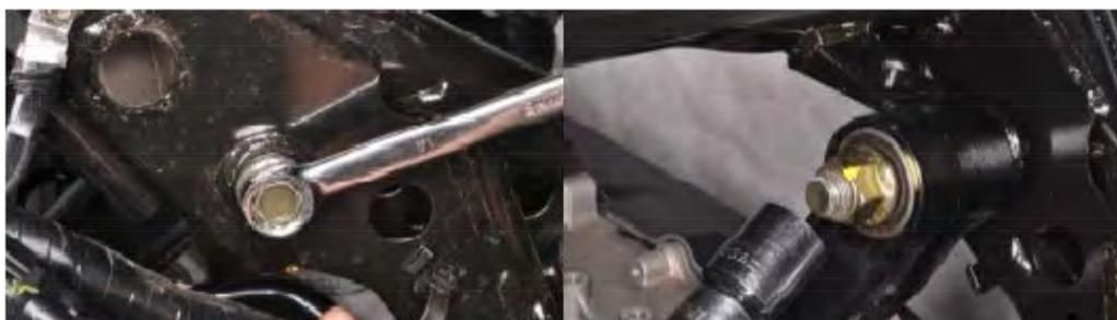
Hold the engine mounting bolts with a 14 mm wrench and loosen the nuts with a 19 mm socket.
