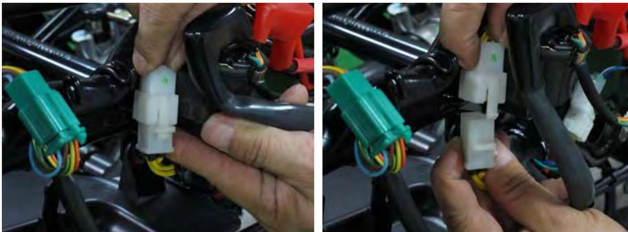
Disconnect the generator 3-pin connector.
