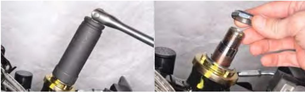
A special lock nut wrench is needed to loosen the steering stem lock nut. Remove the steering stem lock nut. Special Tool - Long Socket Wrench: A120F00007
