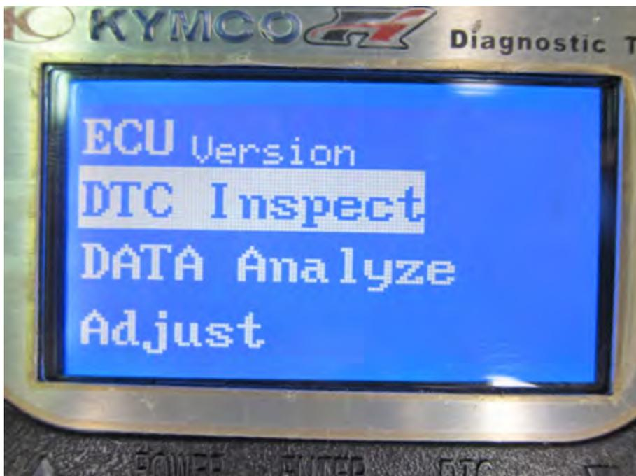
Press the down button (right) to move the item selector down to the DTC Inspect item.
