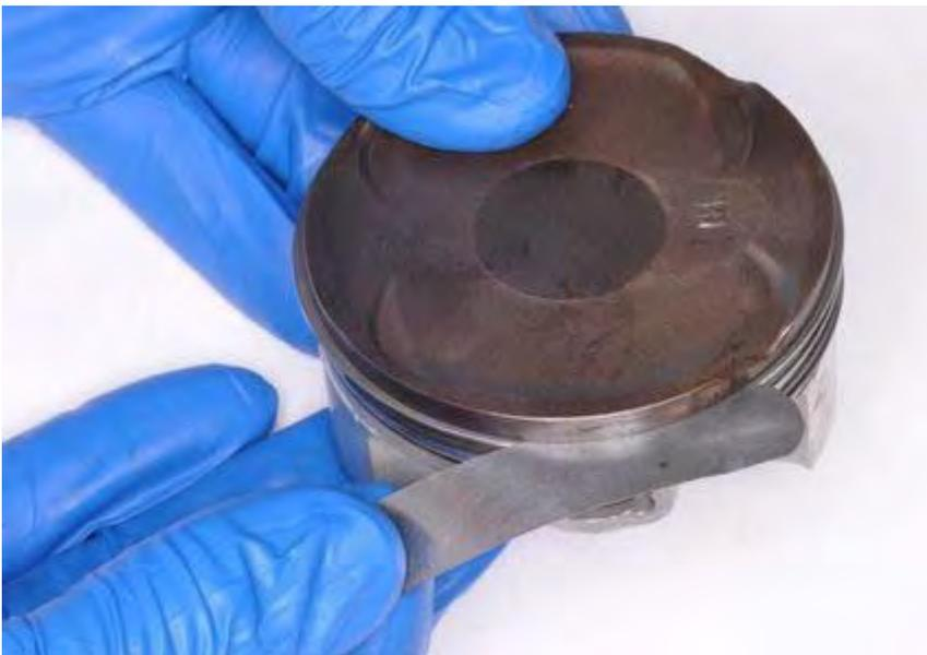
Measure the ring groove width and the ring-to-groove clearance with feeler gauges.
