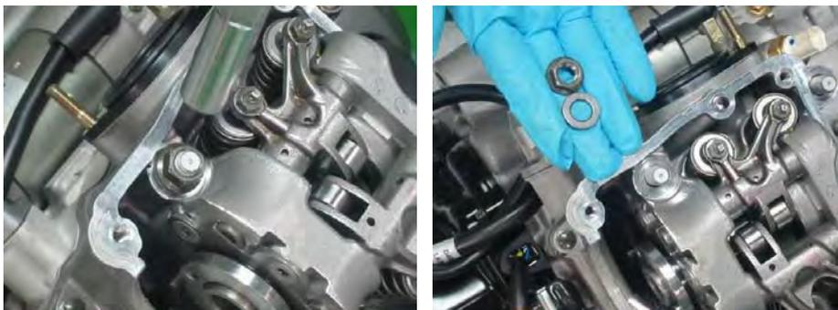
Remove the two nuts and washers on the top with a 14mm socket.
