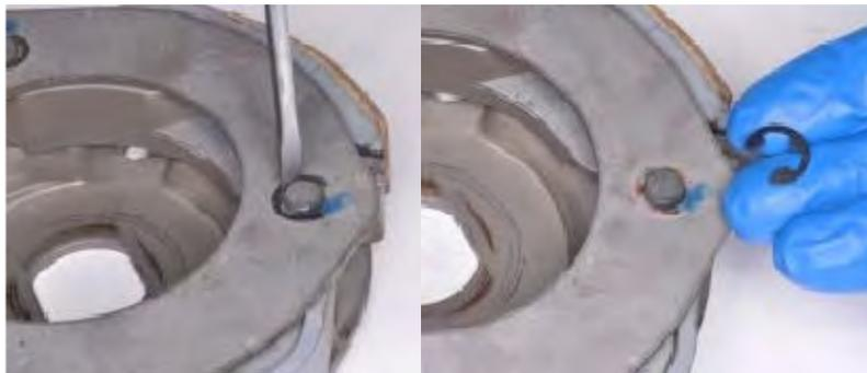
Remove the three circlips from the clutch pivot pins with a small flat blade screwdriver.
