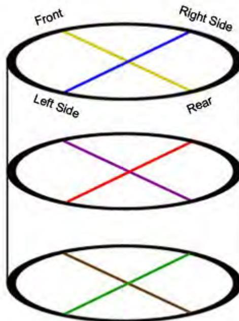
Inspect the cylinder front to back and side to side at three different height levels with a dial bore gauge.
