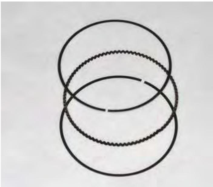
Install the oil expander ring so that the ends are not overlapping. Install the steel rails above and below the oil ring.
