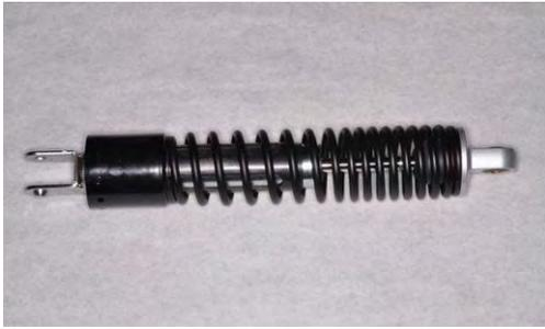
Check over the shock absorber for damage and oil leaks. Replace the shock absorber if needed. Do not attempt to disassemble the shock absorber.
