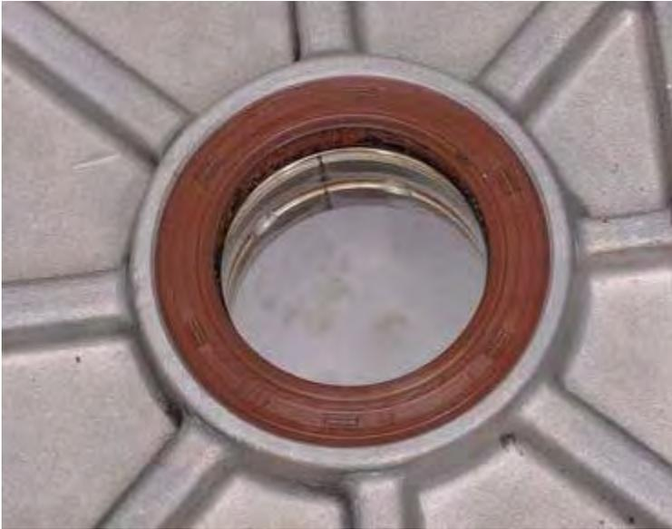
Replace the left crankshaft seal if the crankcases are separated.
