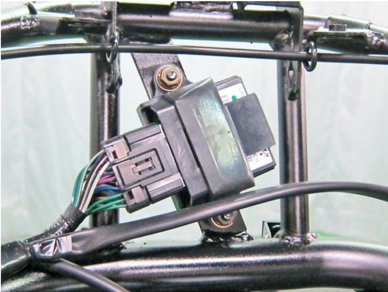
Remove the nuts and bracket to remove the ECU.
