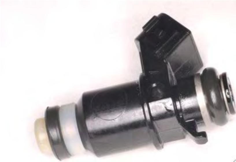
Apply a light coat of fresh engine oil to a new fuel injector O-ring.
