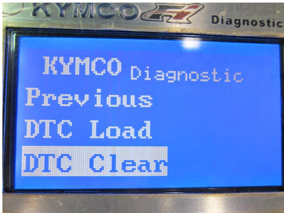
Move the selector down to the Clear DTC option and press enter.
