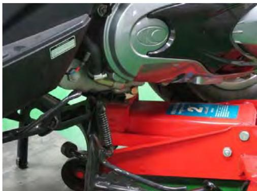
Support the engine with a suitable jack or stand.
