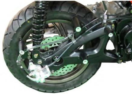
Install the lower shock absorber mounting bolts and torque them to specification with a 14 mm socket.
