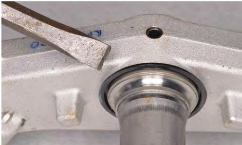
Use a chisel and hammer to drive out the bearing races. Do not damage the frame pipe and steering stem. Have the drift set against the lip of the race, and work around the race evenly to drive it out. Repeat the process with the remaining bearing race.
