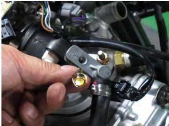
Remove the fuel injector mounting bolt with a 10 mm socket. Unplug the fuel injector connector.
