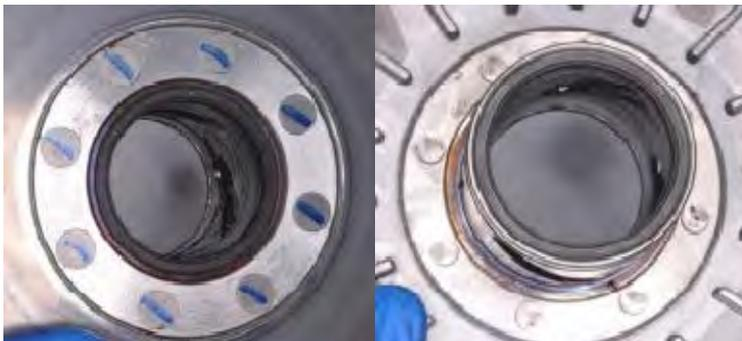
Drive in the new seals with a suitable driver with the same outside diameter as the seal.
