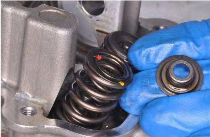
Place the spring retainer on top of the spring.
