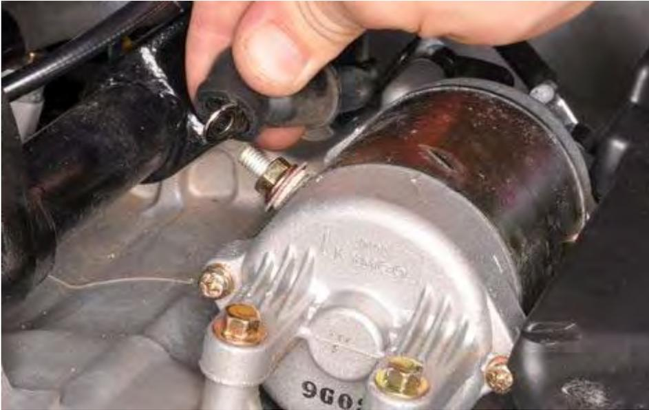
Remove the starter motor lead nut with a 10 mm wrench. Free the cable lead from the starter motor. Thread the nut back on to keep track of it.
