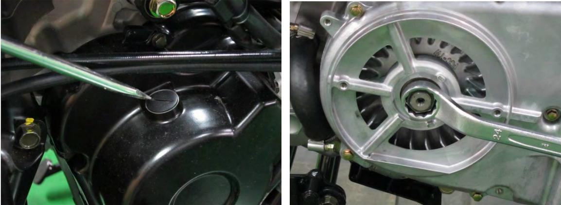
Rotate the crankshaft to TDC mark.
