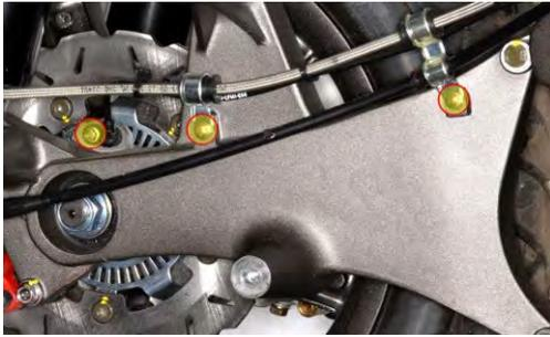
Install the rear wheel speed sensor and hose clamp bolts with an 8 mm socket.
