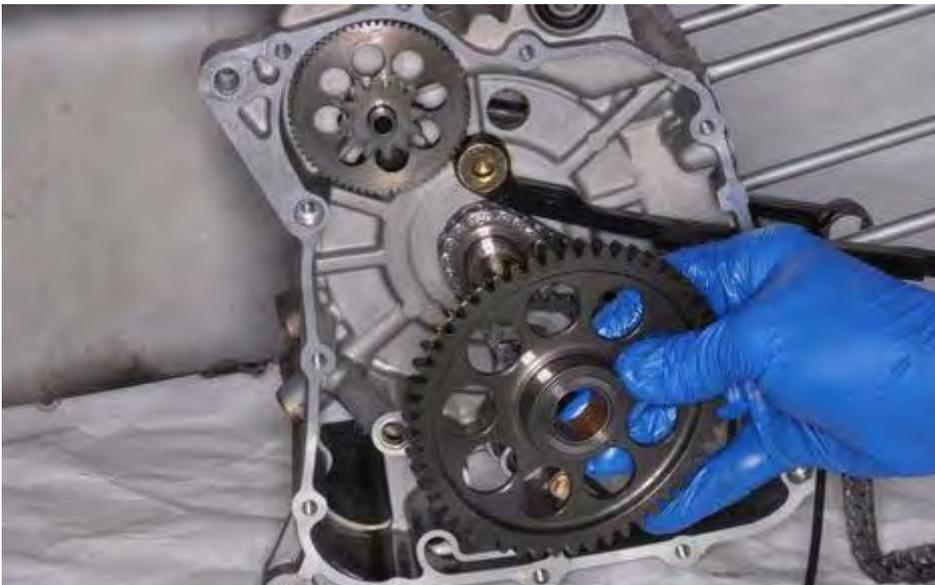
Lubricate the inside of the starter driven gear with fresh engine oil. Slide the starter driven gear onto the flywheel as shown.
