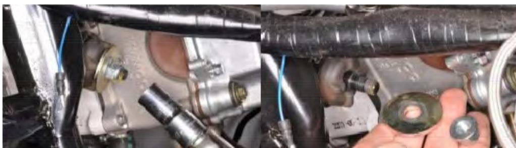
Loosen the engine mounting bracket damper nut with a 14 mm socket.
