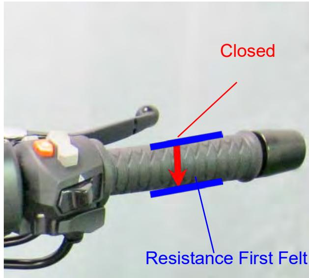
Check the throttle cable free play by gently rotating the throttle grip back until resistance is felt.
