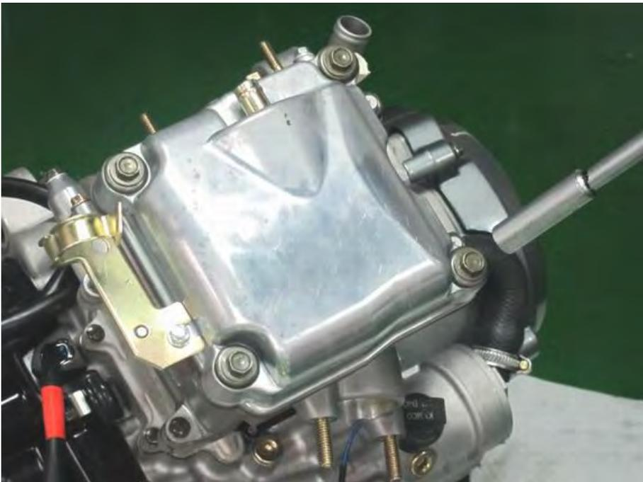
Tighten the cylinder head cover bolts securely in two steps and in a crisscross pattern with an 10 mm socket.
