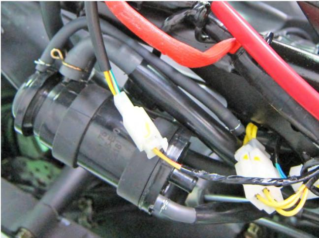
NOTE: The tube should not be wrenched or crashed and never refit the canister.
