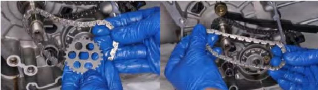
Inspect the oil pump drive chain and sprocket for signs of wear and damage. Replace the parts as needed.
