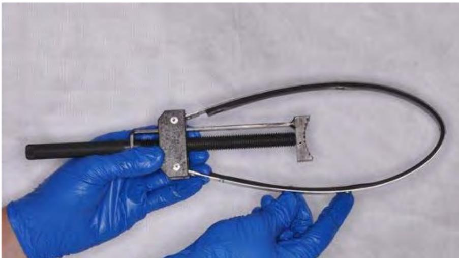
To remove the fly wheel two special tools are needed.
