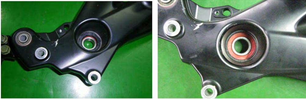
Inspect the wheel bearing by turning it with a finger. Replace the bearing and seal as needed.
