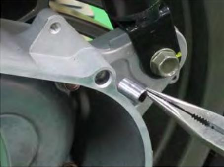
Install the two dowel pins into the belt case.
