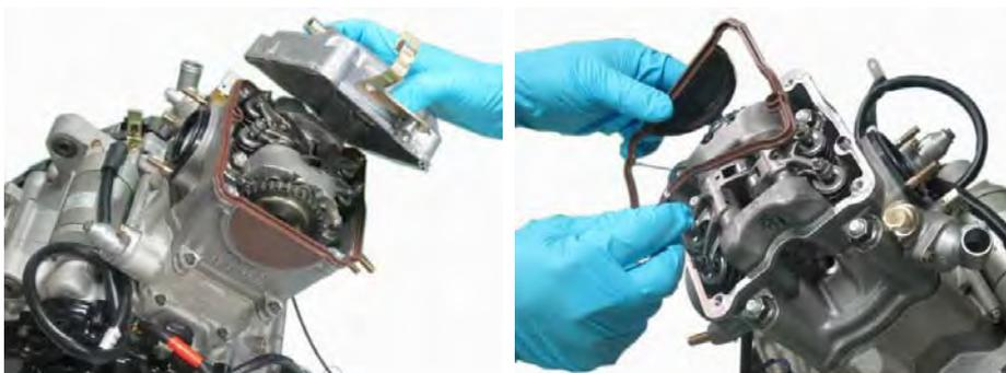
Remove the cylinder head cover and gasket.
