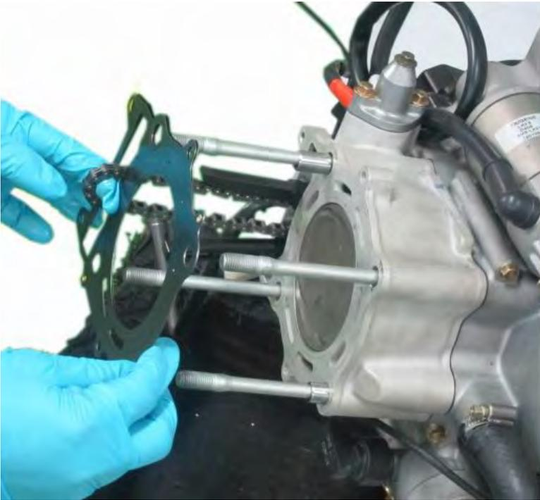
Install the new base gasket onto the crankcase.
