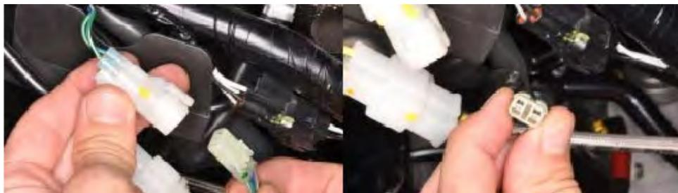
Disconnect the crank position sensor wire coupler.
