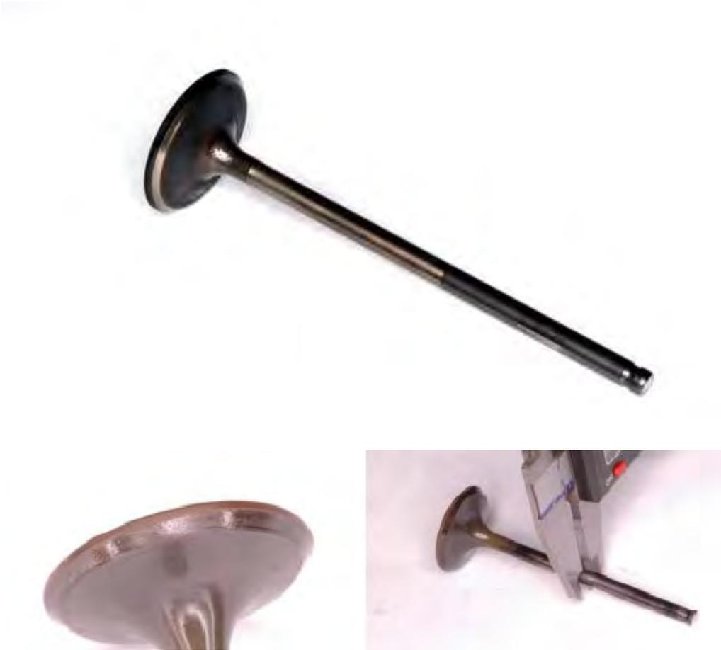
Inspect the valves for damage and burning. Measure the valve stem diameter in several places where the valve makes contact with the guide. If the measurement is below specification replace the valve.
