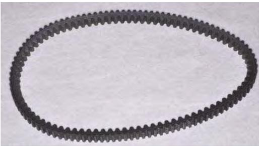
Inspect the drive belt for cracks or excessive wear.
