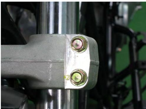
Loosen the lower fork clamp pinch bolts with a 12 mm socket. The top bolts must be removed.
