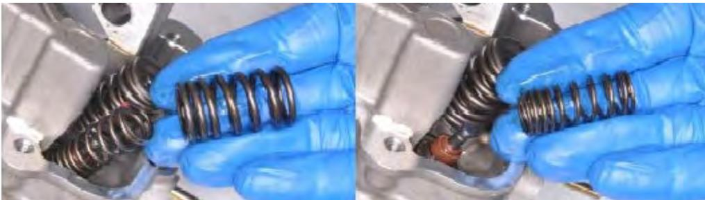
Remove the valve springs.
