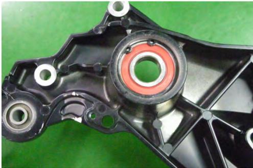
Remove the seal and snap ring.
