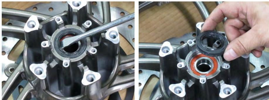
Remove the dust seals from the each side of the front wheel using a seal pick or large flat blade screwdriver. Discard the dust seal, it should be replaced by a new item.
