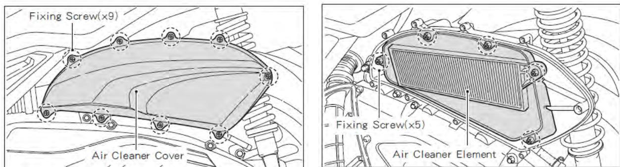
The new air cleaner element set installation is in the reverse order of removal.
