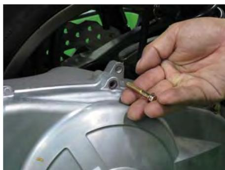
Remove 11 the belt case cover bolts with an 8 mm socket.
