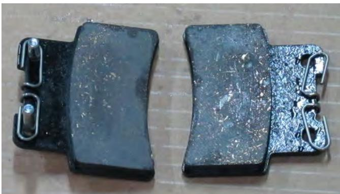
Replace the pads if the brake wear exceeds the wear indicator lines or if the wear is uneven.
