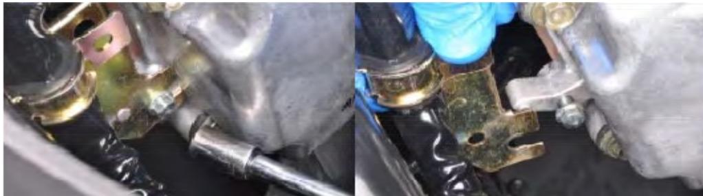
Loosen the fuel hose stay bolt with an 8 mm socket. Free the fuel hose stay from the cylinder head cover.
