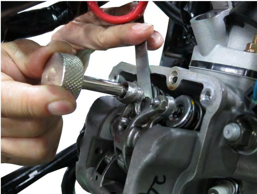
Place a 9 mm box end wrench over the locknut, and loosen the locknut. If the valve clearance is tight back out the valve tappet adjusting screws with the tappet adjustment tool. If the clearance is to loose turn in the adjusting screw until there is a light drag on the feeler gauge. Hold the adjusting screw locknut in place with the wrench to make sure it doesn't interfere with the adjustment.
