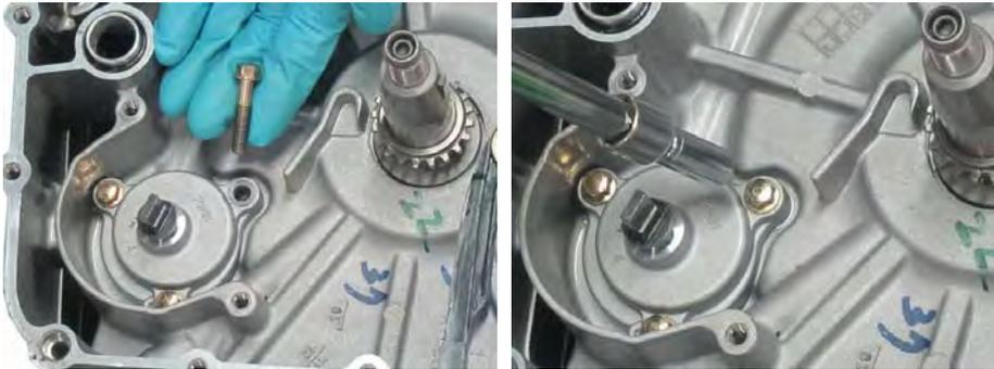
Insert the three oil pump mounting screws and tighten them securely with an 8mm socket.
