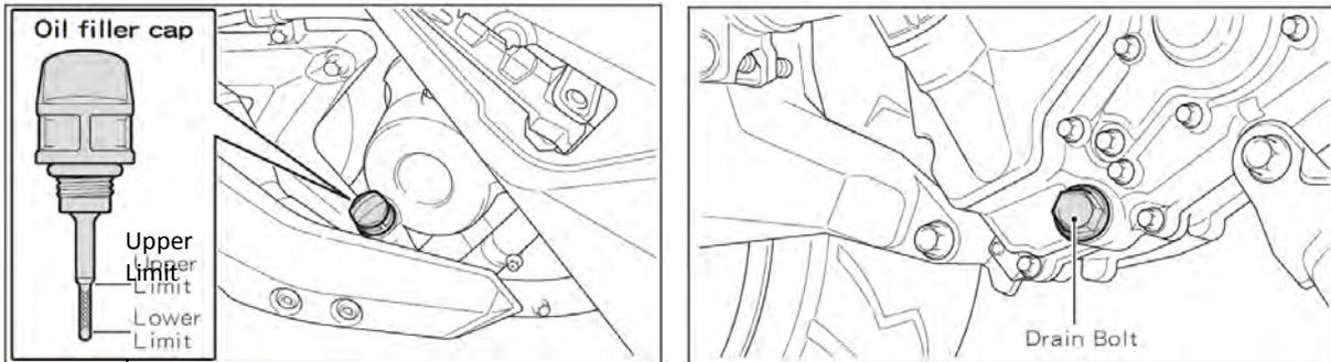
3. Fill in new oil. Filling capacity is 1.5L.
