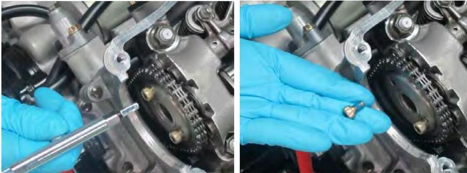
Use a 5 mm Allen wrench to remove the camshaft sprocket bolts.
