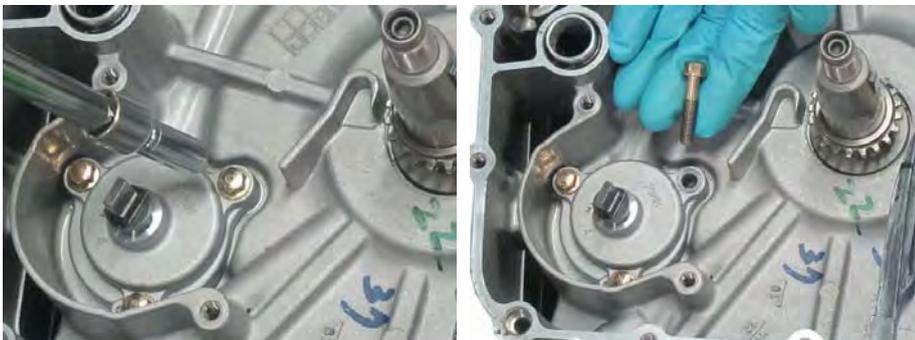
Remove the three oil pump screws with an 8mm socket.
