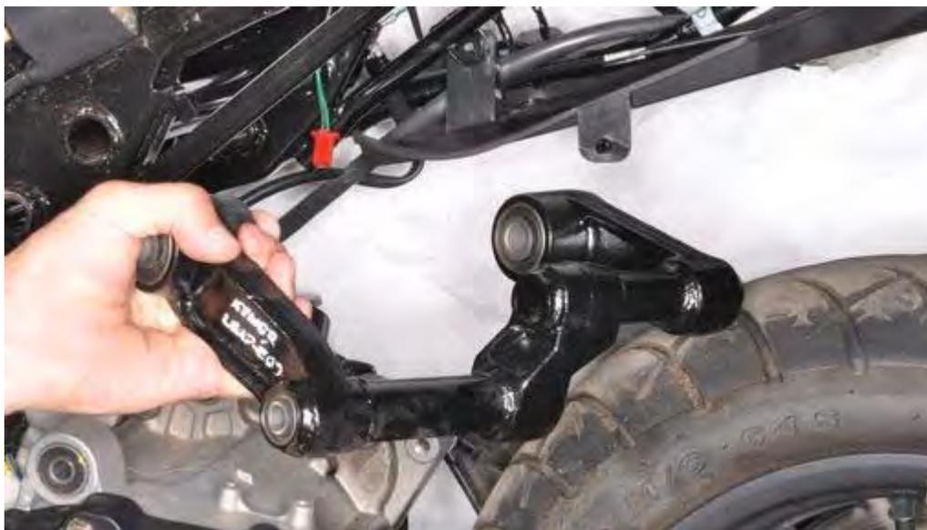
Remove the engine mounting bracket.
