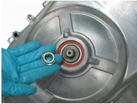
Remove the #M14 nut mounting the clutch outer.
