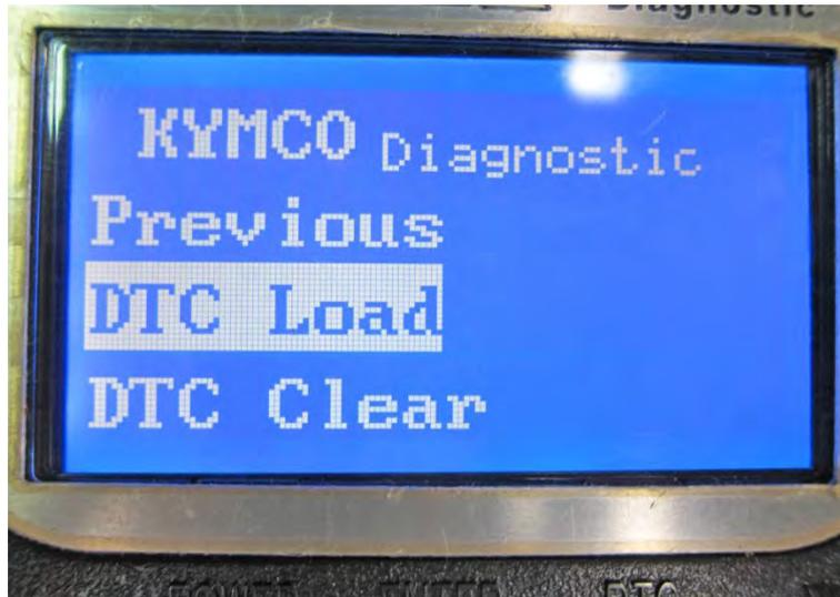
Press the down button (right) to move the item selector down to the DTC Inspect item.
