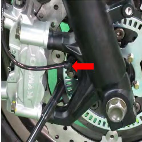
Remove the front wheel speed sensor mounting bolt with an 8 mm socket. Free the front wheel speed sensor from the right fork.
