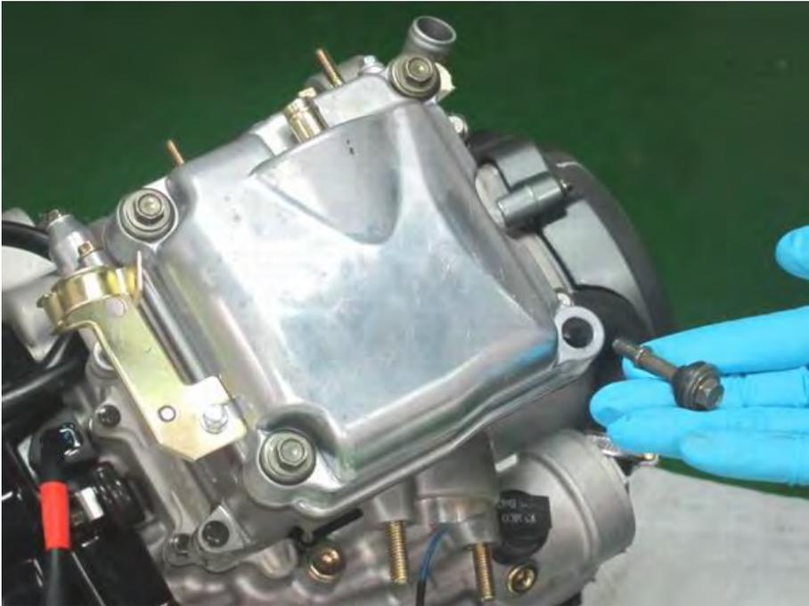
Coat the cylinder head cover bolt seals in fresh engine oil. Insert the cylinder head cover bolts with grommet seals and washers. Note the gold colored and longer bolts go on the right side.
