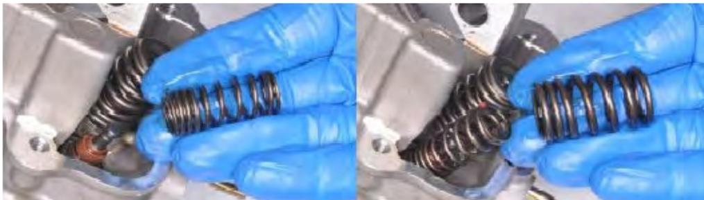
Install the valve springs. The tightly coiled end of the springs should sit against the spring seat.
