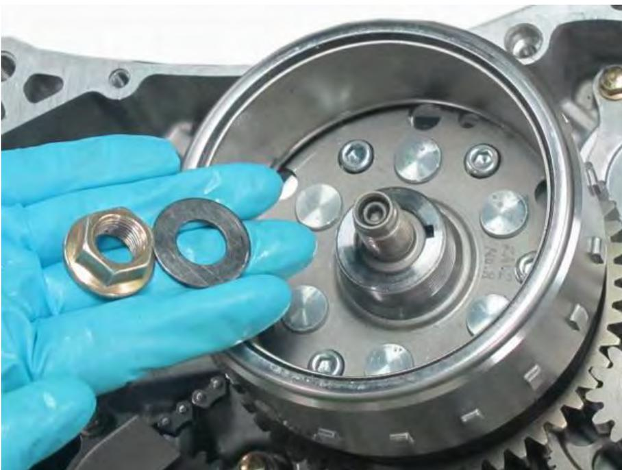
Install the washer and flywheel nut.
