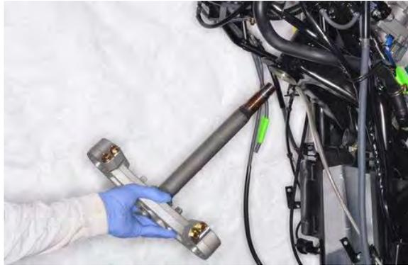
Lift out the upper ball bearings. And slide the lower ball bearings up and off of the steering stem.
