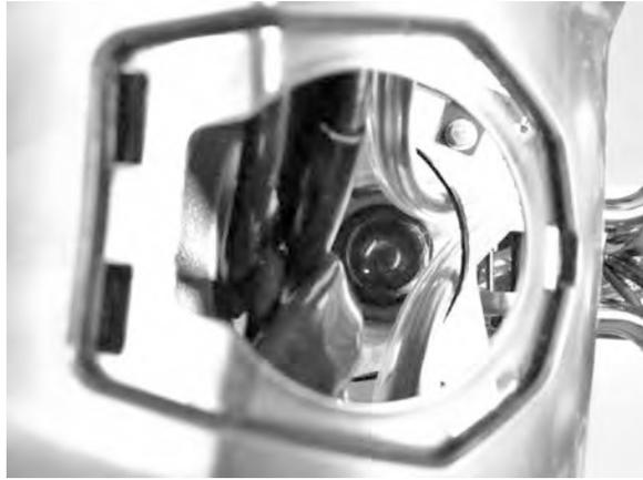
Remove the bolts, screws.
