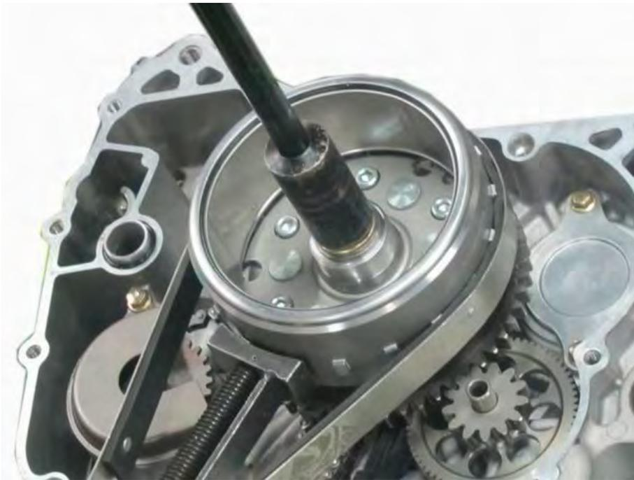
Hold the flywheel with the universal holder and torque the flywheel nut to specification with a 19 mm socket.
