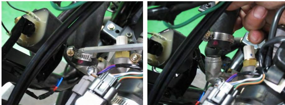
Loosen the thermostat hose clamp with a #2 Phillips screwdriver.
