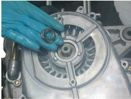
Remove the #M18 nut mounting the drive face.
