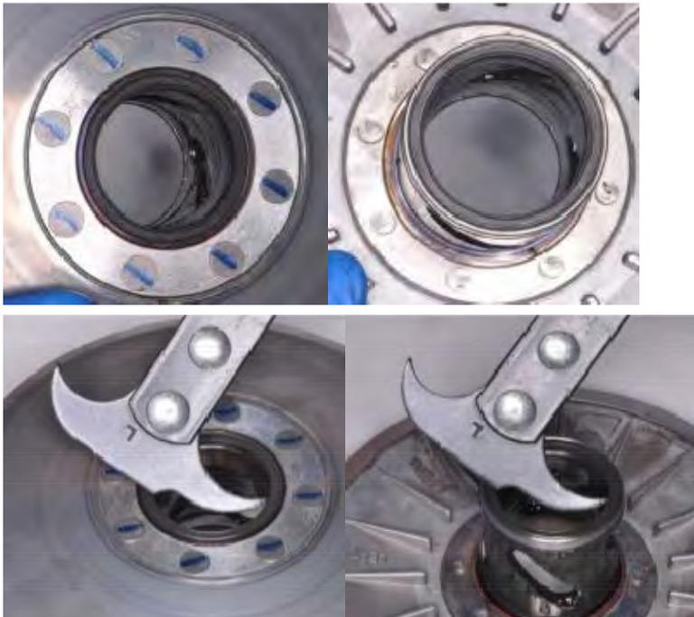
Remove the seals from the left face of the driven pulley.
