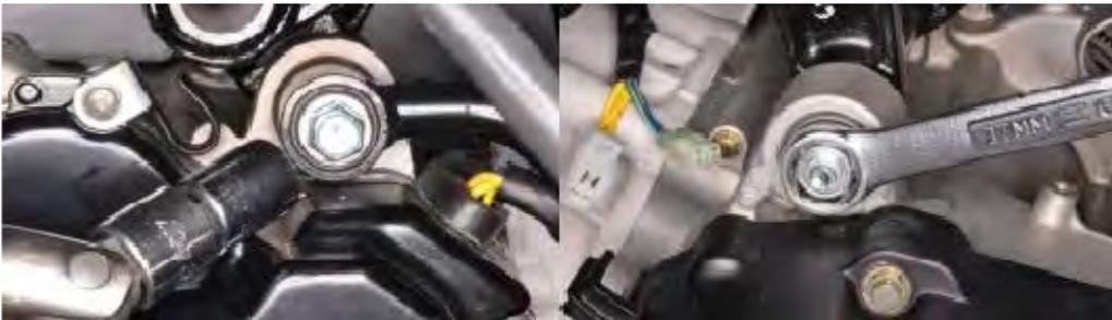
Loosen the engine mounting bracket damper bolt and nut with a 17 mm wrench for the nut and a 14 mm socket for the bolt.
