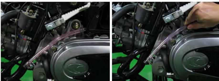
Disconnect the drain hose from the air cleaner.
