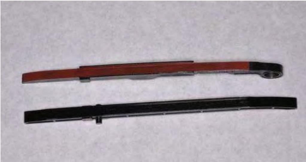
Inspect the cam chain guides for damage and excessive wear. Replace the guides as needed.
