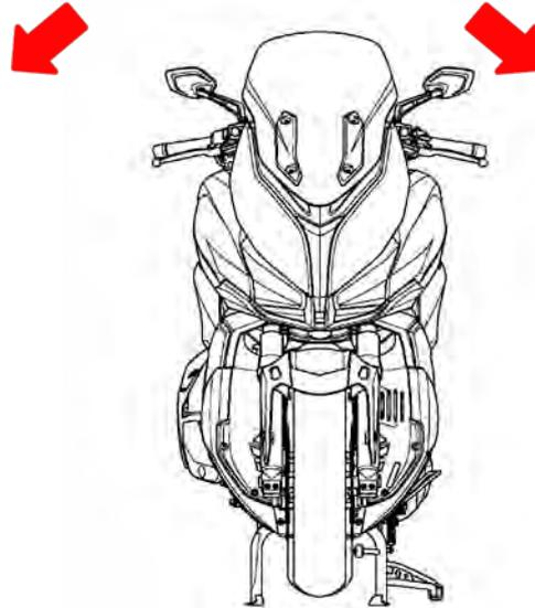
Raise the front wheel off the ground and check that the steering handlebar rotates freely. If the handlebar moves unevenly, binds, or has vertical movement, adjust the steering head bearing. See the Steering Stem Removal topic for more information.
