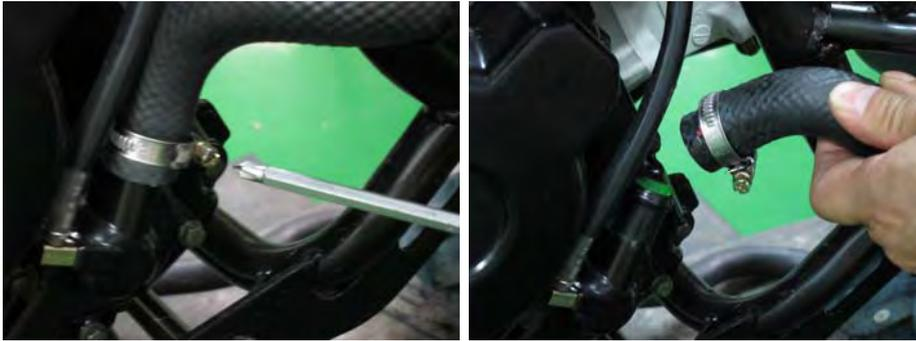
Loosen the water pump hose clamp with a #2 Phillips screwdriver. Slide up the clamp and free the coolant hose from the water pump. Allow any remaining coolant to drain into a suitable container.
