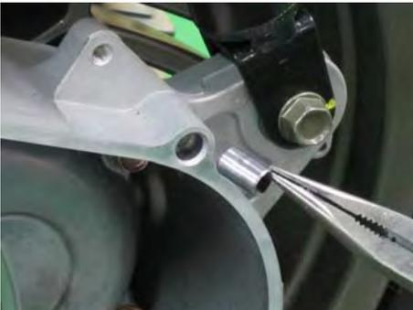
Remove the two dowel pins.
