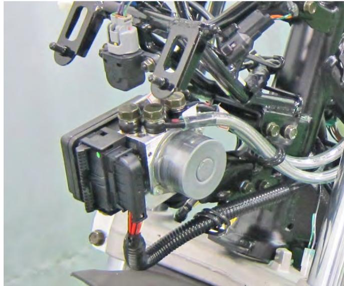
Note the markings on the ABS unit for the brake Front (F) and Rear (R) brake hose positions.
