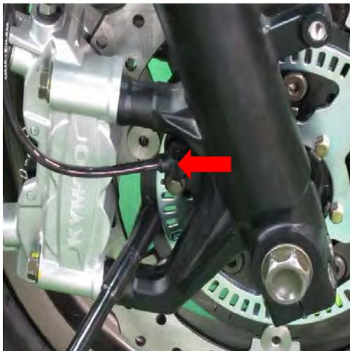
Install the speed sensor and its mounting bolt to the right fork leg. Tighten it securely with an 8 mm socket.
