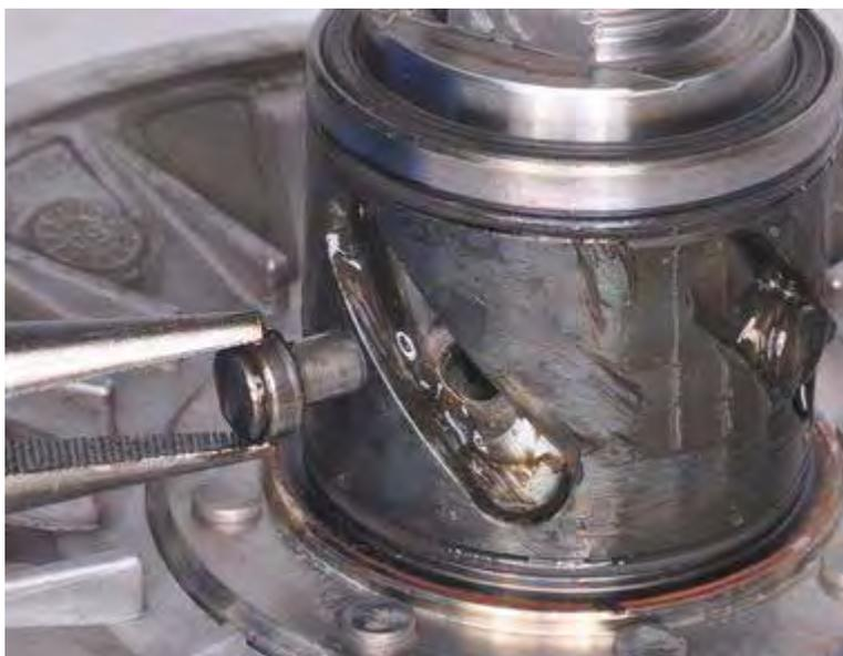
Remove the four guide rollers with guide roller pins.
