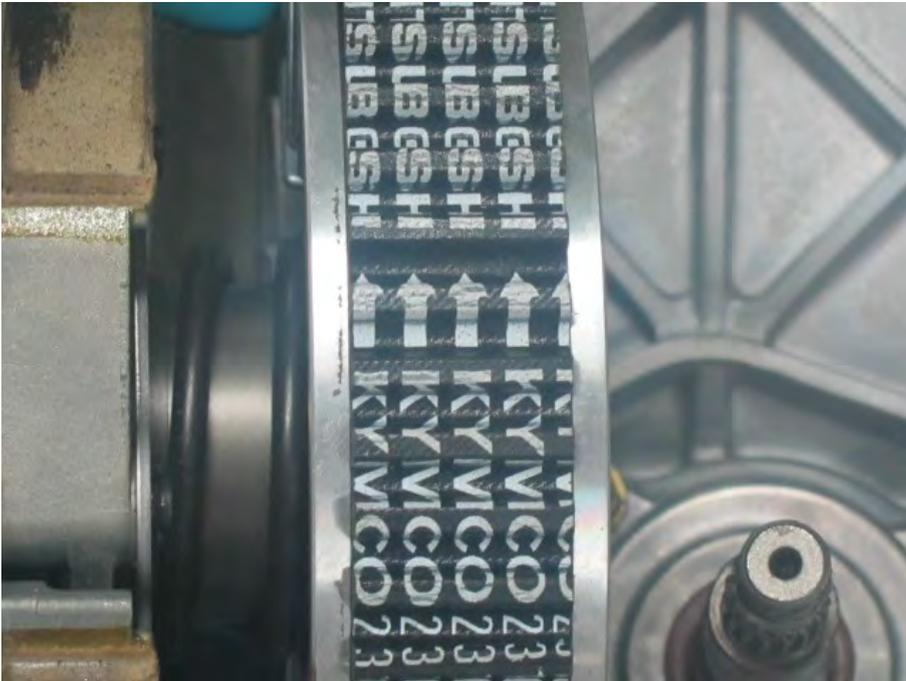
Inspect the drive belt for cracks or excessive wear.
