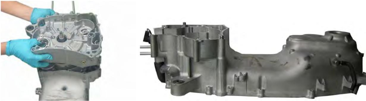
Set the right case half down on top of the left. Install the engine mount spacer.
