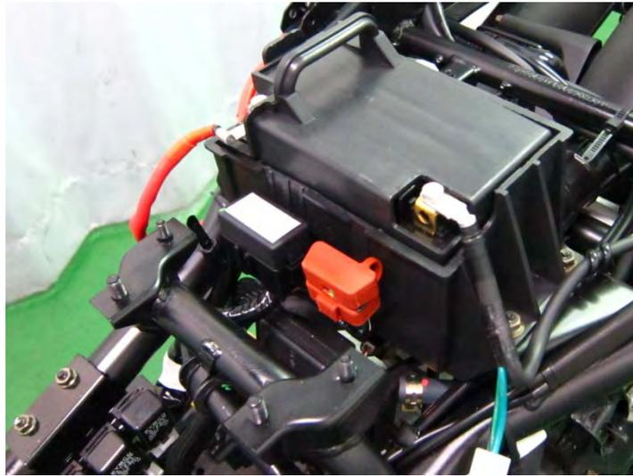
Use the Sub cord, OBD diagnostics connector (part number:36205-LGC6-E00) to connect between vehicle and diagnostic tool.
