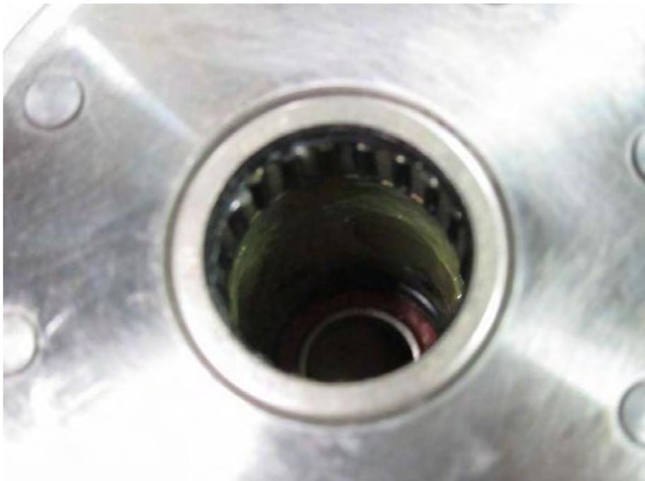
Inspect the bearings in the right face of the driven pulley.
