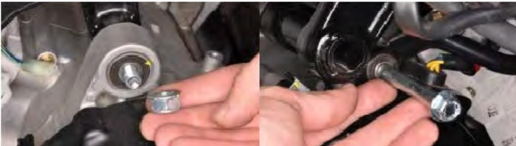
Remove the engine mounting bracket damper bolt and nut.
