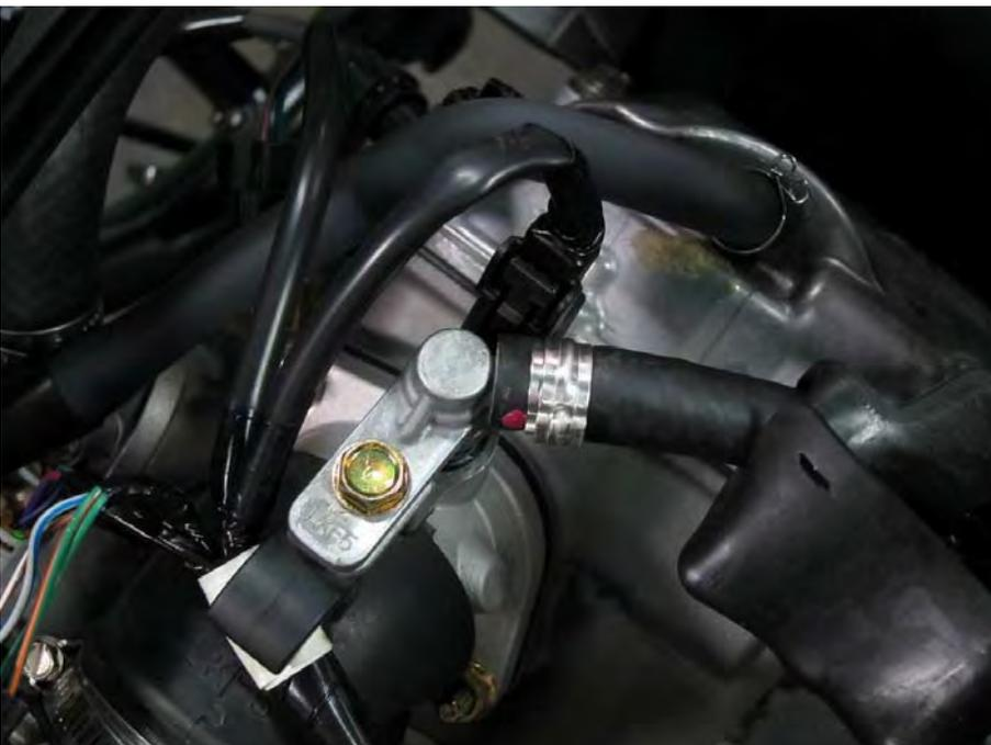
Free the wiring harness from its guide above the intake pipe.
