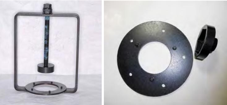
Fit the clutch and fitting tool into the clutch spring compressor tool.
