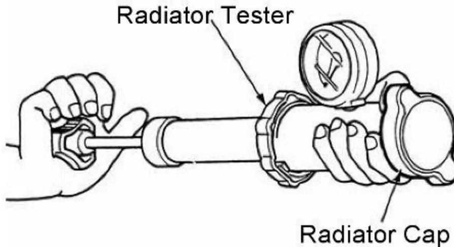
Wet the seal on the radiator cap and install it to the pressure tester.
