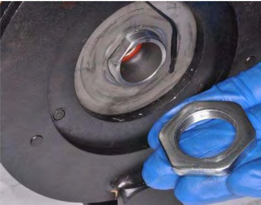
Remove the clutch drive plate nut.
