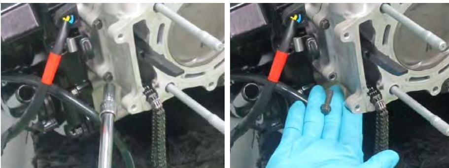
Remove the two cylinder bolts on the right side of the engine.
