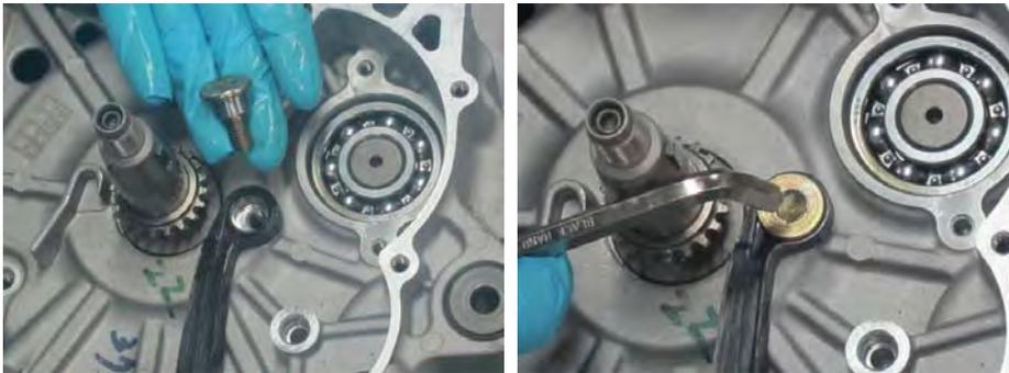
Fit the upper cam chain guide into place.
