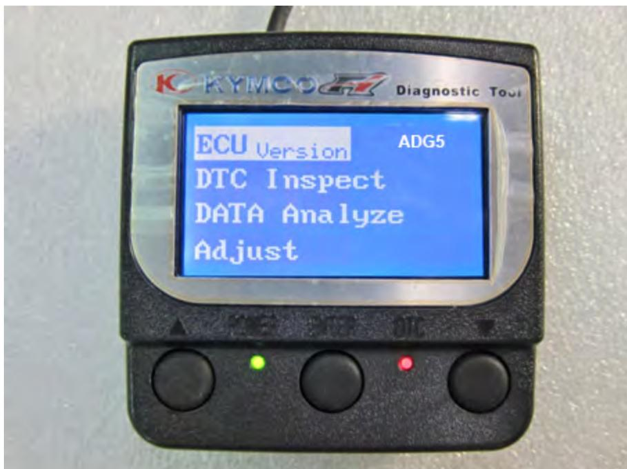
The four functions will display when the tool is powered on. The model name will show ADG5 for the XCITING S 400.
