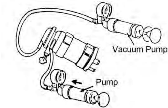
NOTE: Always using the pump by manual, do not apply high pressure for testing to prevent the valve from malfunction.
