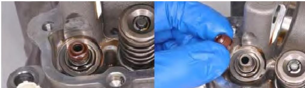
Remove the valve seal from the valve guide. The valve seals should be replaced if they are removed or you are going to install new valves.
