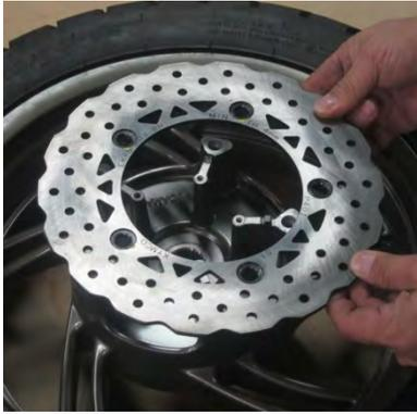
Lift off the rear brake disc.
