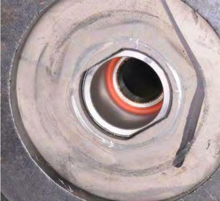
Inspect the left side bearing by turning it with a finger. If the bearing is rough turning or noisy it should be replaced.
