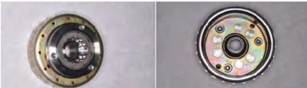
Fit the starter clutch to the back of the flywheel. Apply blue Loctite to the threads of the three starter clutch mounting bolts. Insert the three starter clutch mounting bolts.
