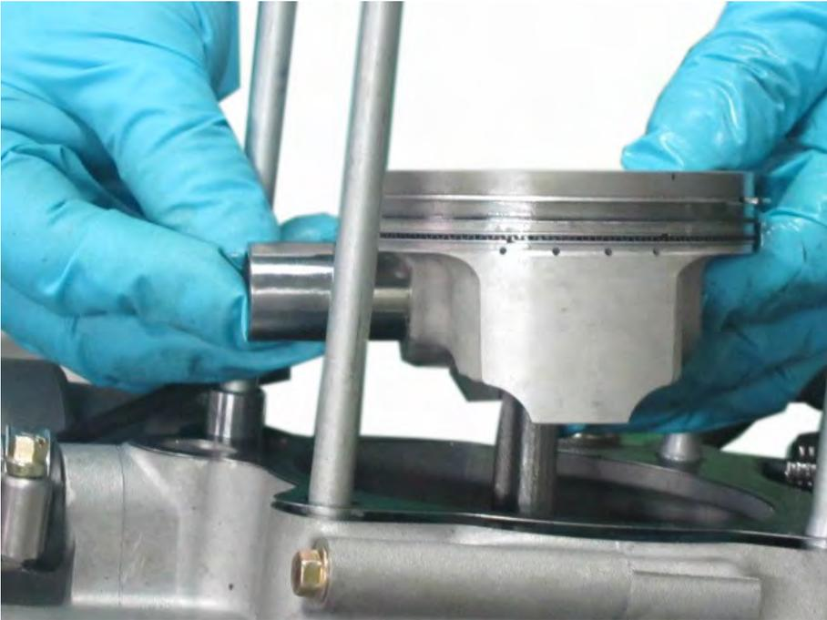
Remove the piston pin and the piston.
