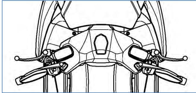
Pump the brake lever several times and hold the lever in. While holding the lever in, crack open the bleeder valve. The front brake lever will travel all the way to the grip and brake fluid and/or air will come out of the bleeder valve into the 6 mm hose. Tighten the bleeder valve before releasing the front brake lever. Pump the lever several times again and repeat the process.
