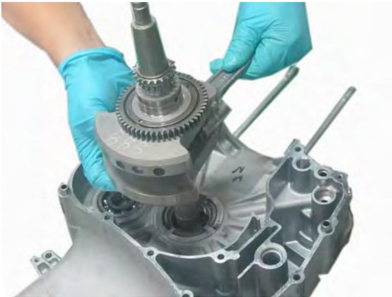
Lift the crankshaft out of the left crankcase half.
