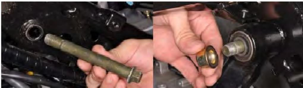
Install the two engine mounting bracket to frame mounting bolts and nuts. Insert the bolts from the outside of the frame.
