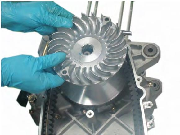
Remove the left face of the drive pulley.
