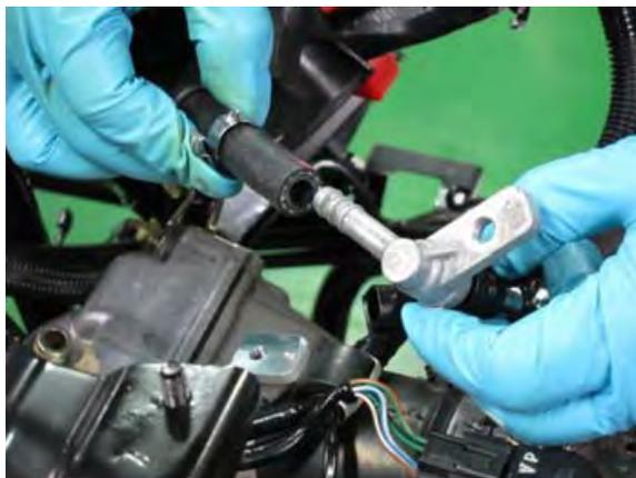
Slide back the clamp and free the injector fuel pipe from the fuel hose.
