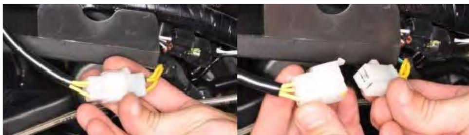
Disconnect the generator 3-pin connector.
