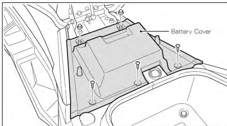
Remove the negative battery cable bolt and free the negative cable from the battery first. Then remove the positive battery cable bolt and lift the battery out of the battery tray.
