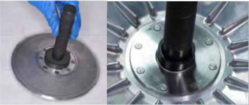
Drive in the new seals with a suitable driver with the same outside diameter as the seal.
