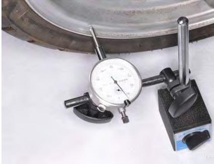
Place the wheel on a truing stand and use a dial indicator to check if the rim is out of true. The specifications for the front and rear wheels are the same. Check for lateral wobble. The service limit is 2.0 mm (0.08 in) or less.
