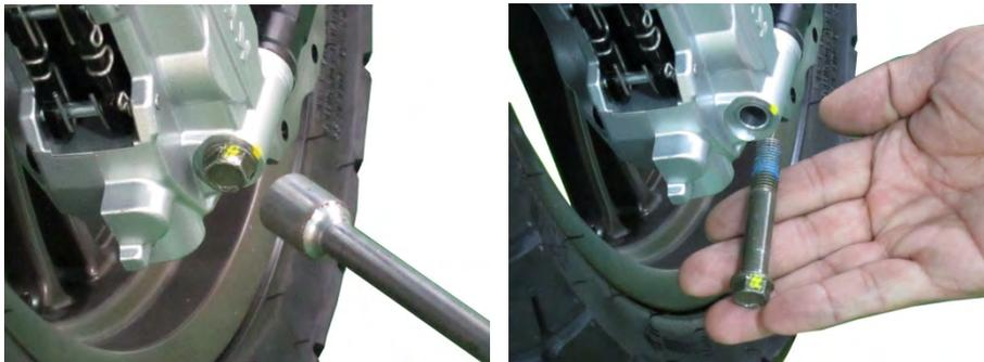
Remove the two caliper mounting bolts with a 12 mm socket. Discard the brake caliper mounting bolts.
