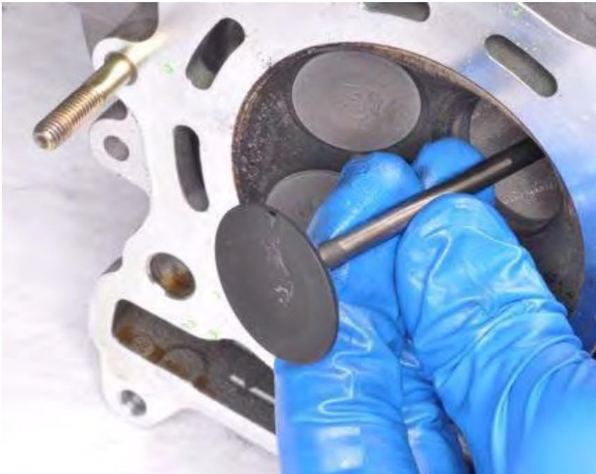
Coat the valve stem in fresh engine oil and insert the valve into the valve guide and through the seal. Turn the valve slowly as it is inserted. If you are installing a new valve you must ream the valve guide first. Make sure the valve will move smoothly in the valve guide without wobble.
