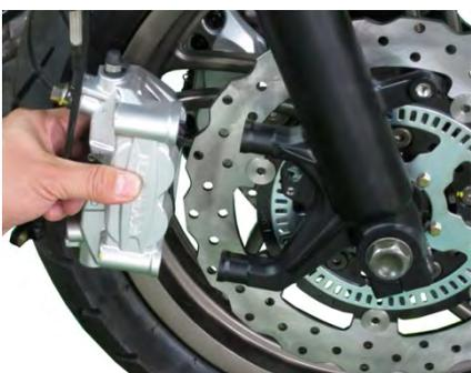
Remove the front brake caliper.
