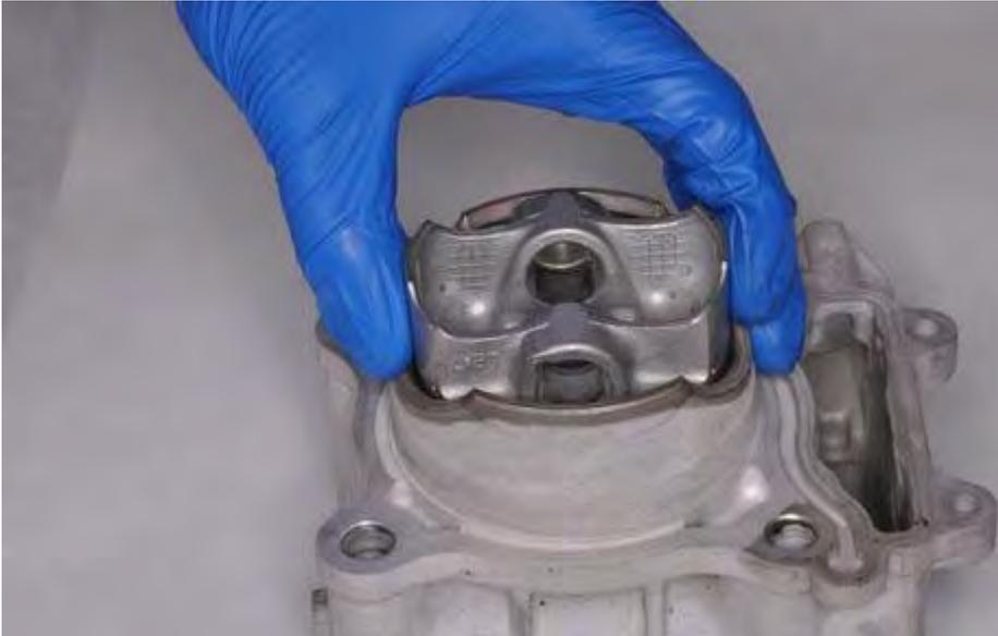
Insert the top ring into the cylinder. Push the top ring in the cylinder about an inch. Use the piston to push in the ring to keep it square with the cylinder.
