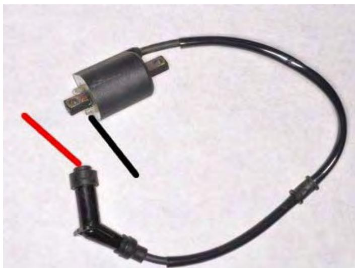
Check the secondary resistance between the ignition coil terminal and the spark plug cap. Touch the negative meter lead to the terminal and the positive meter lead to the spark plug cap as shown.
