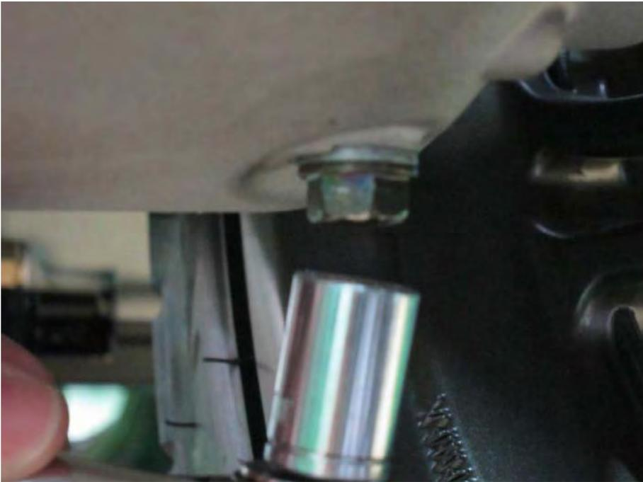
Install the oil drain plug and washer with a 12 mm socket.
