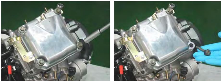
Loosen the four cylinder head cover bolts with a 10 mm socket.
