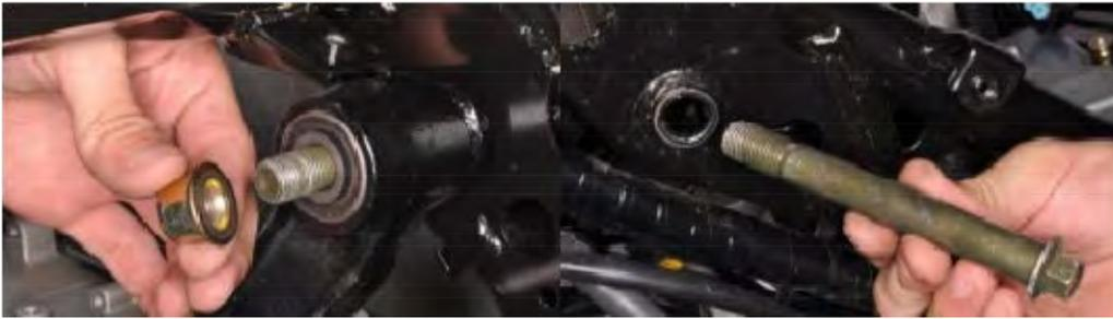
Remove the engine mounting nuts and bolts from both sides.
