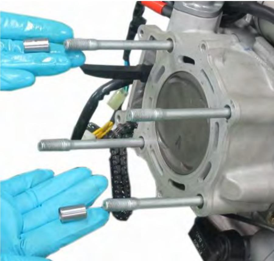
Remove the two cylinder dowel pins from the left studs.
