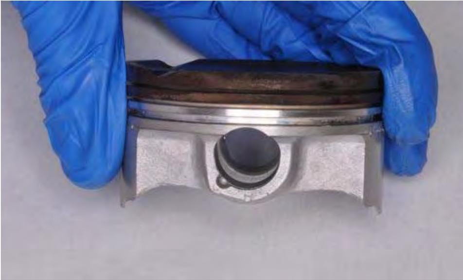
Also clean out the ring grooves. You can use an old ring to scrape out any carbon build up in the grooves.
