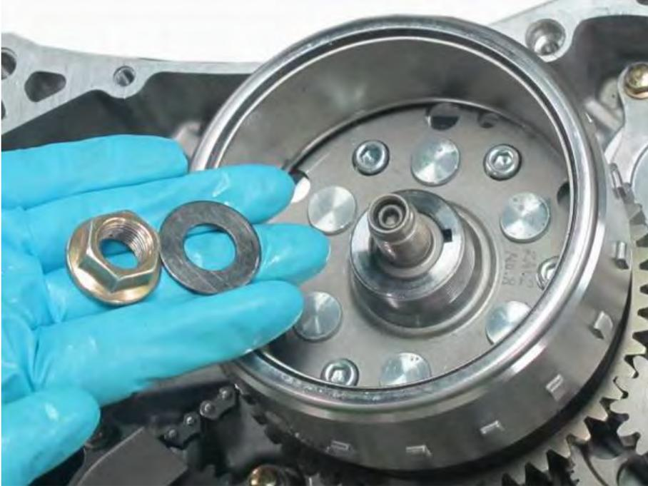
Remove the flywheel nut and washer.
