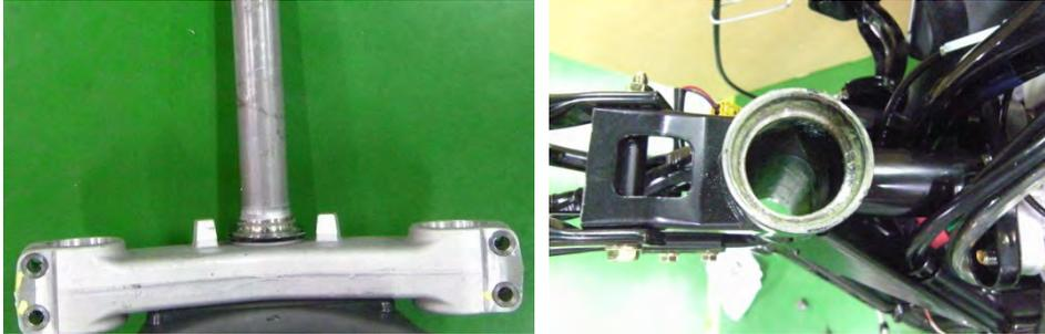
Inspect the bearings and races for wear and damage.
