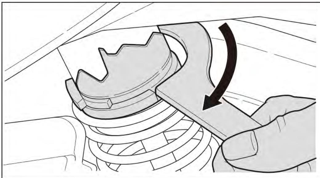
Use a pin spanner to adjust the rear shock spring preload. The shock absorbers are adjustable for pre-load. There are 5 settings. Position 1 is the softest and 5 is the stiffest.
