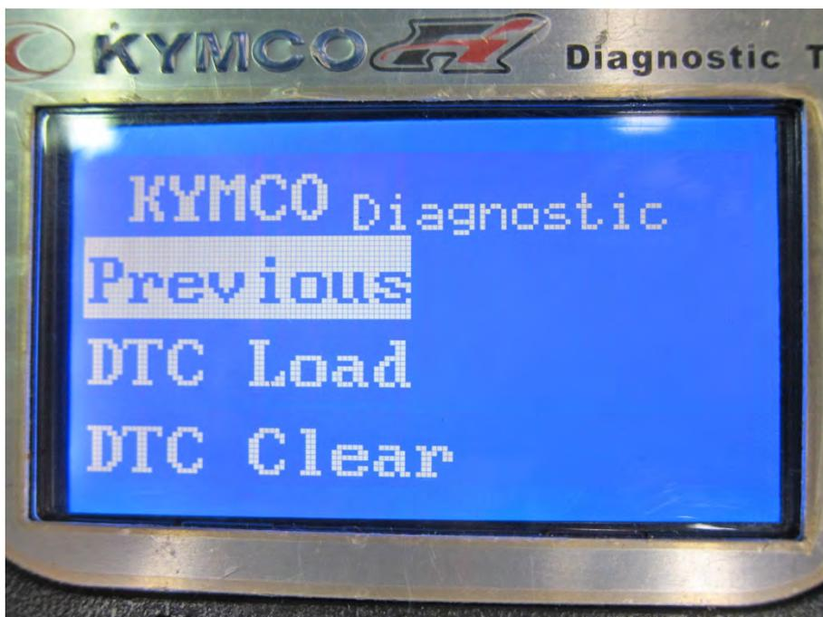
Pressing the enter button on the DTC Inspect item will bring up the options shown above.
