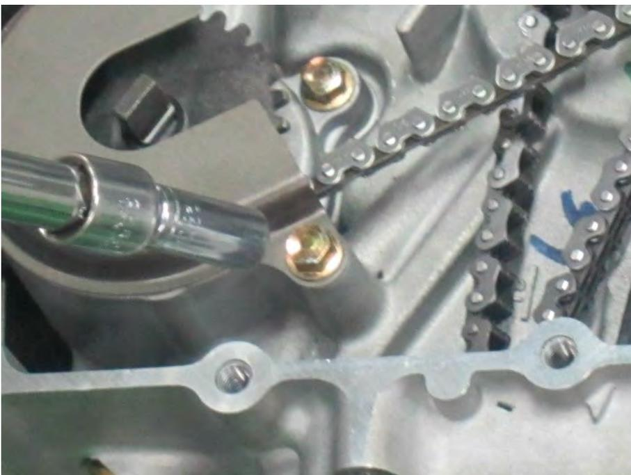
Loosen the two oil pump cover bolts with an 8 mm socket.
