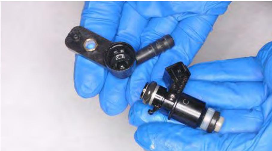
Fit the fuel injector pipe onto the top of the injector. The tab on the injector must fit into the pipe.
