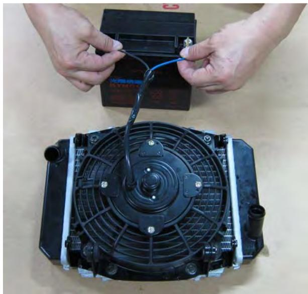
Jump a 12 volt battery to the fan connector and make sure the radiator fan operates.
