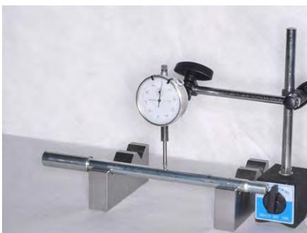
Check the front axle runout. The axle runout specification is half of the total indicator reading. Replace the axle if the measurement exceeds 0.2 mm or 0.008 in.
