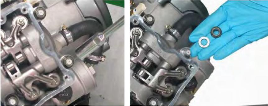
Remove the two nuts and washers on the left side with a 14mm socket.
