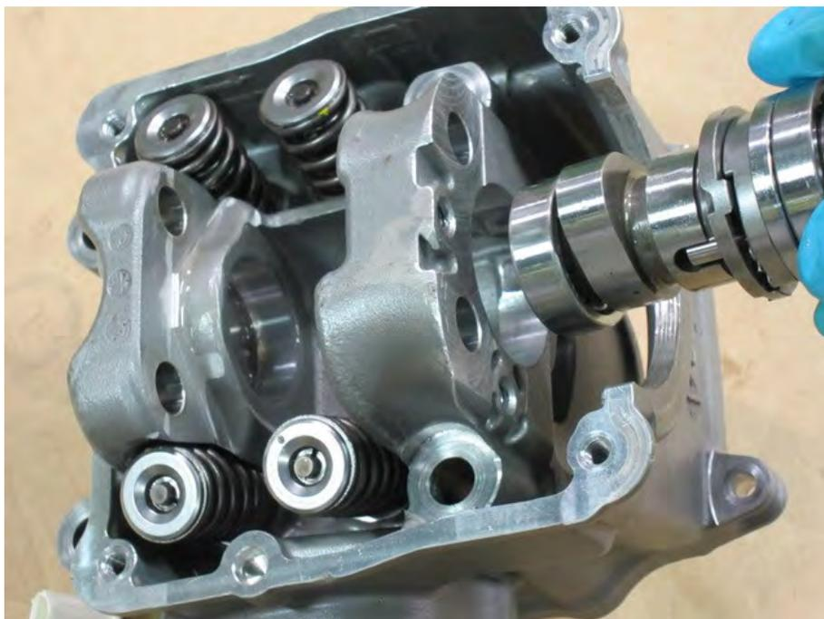
Insert the camshaft into the camshaft holders with the lobes facing down.
