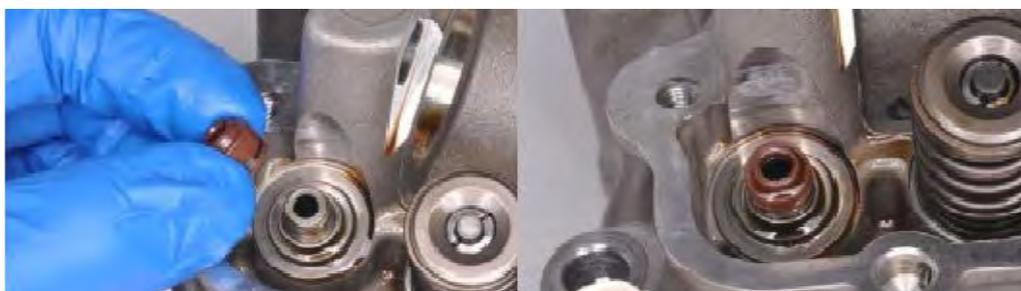
Coat the new valve seal in fresh engine oil and install it onto the valve guide.
