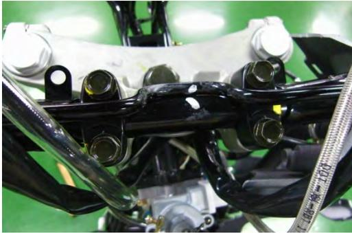
Loosen the four handlebar bolts with a 12 mm socket. Remove the handlebar holders and bolts.
