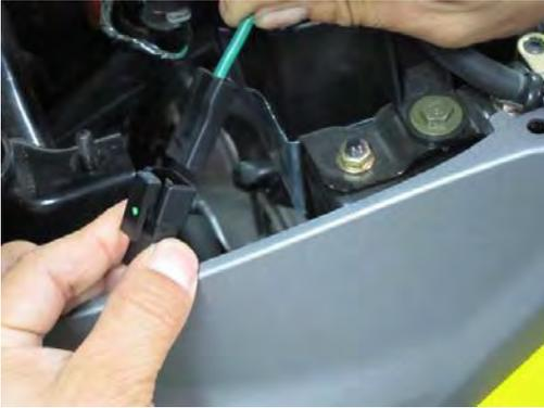
Disconnect the main engine ground wire. Free the engine ground from the left side of the engine.
