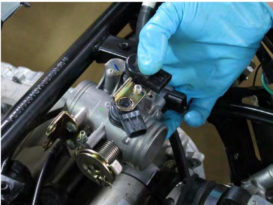
Remove the sensor couplers, remove the throttle out of the air box and intake boots, then remove the throttle body.
