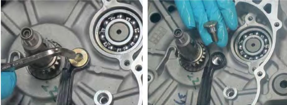
Remove the upper cam chain guide bolt with an 8 mm Allen.
