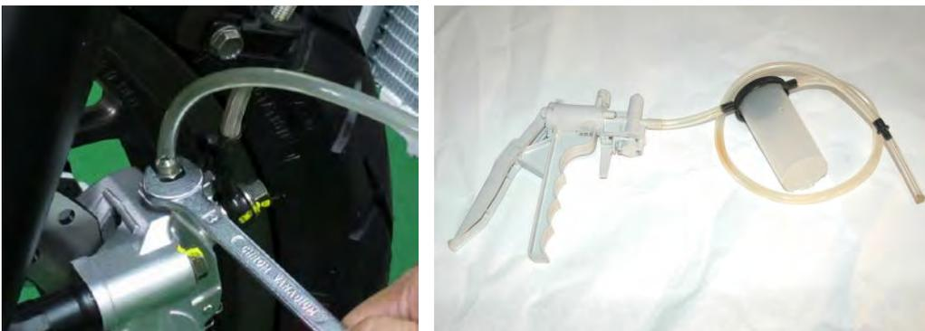
Pull off the rubber cap over the bleeder valve and crack open the bleeder valve on the brake caliper using an 8 mm wrench. This valve is usually very tight so use a box end wrench or a 6 point socket and ratchet to prevent rounding off the head. Snug the bleeder valve back down.
