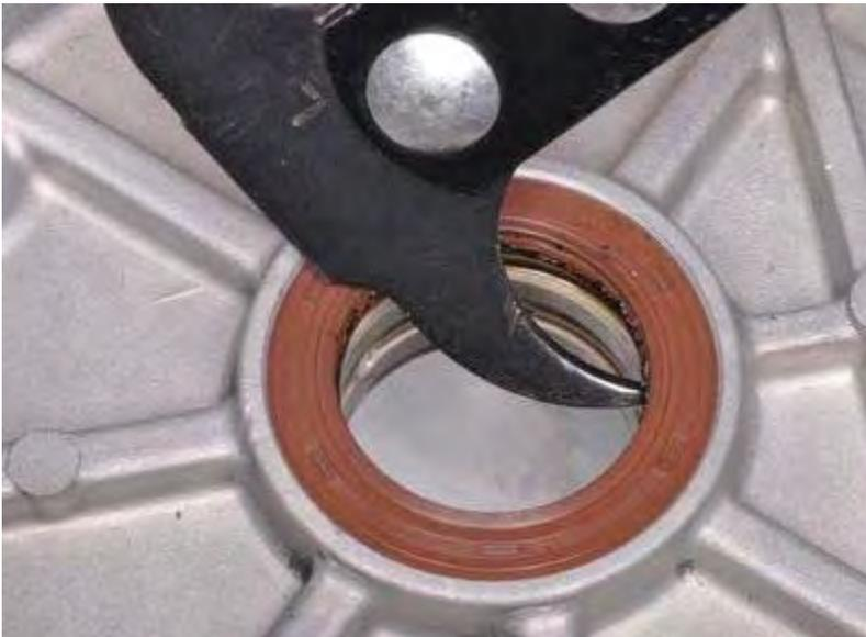
Remove the seal with a seal pick.
