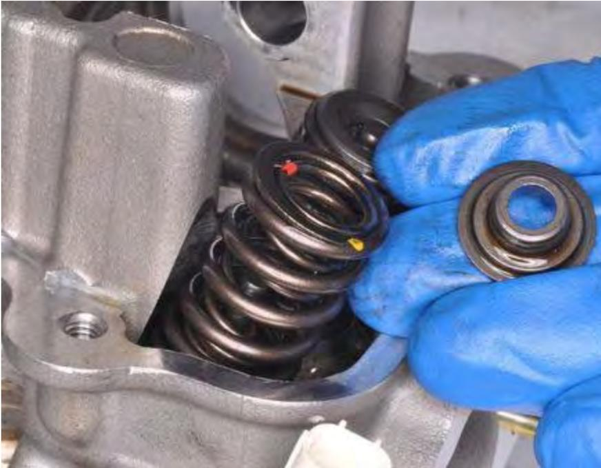
Remove the spring retainer.
