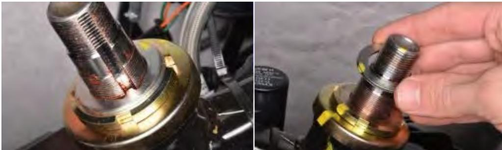
Slide off the lock washer. Loosen the steering stem adjusting nut with the special tool or a pin spanner. Special Tool - Steering Stem Top Thread Wrench: A120F00023
