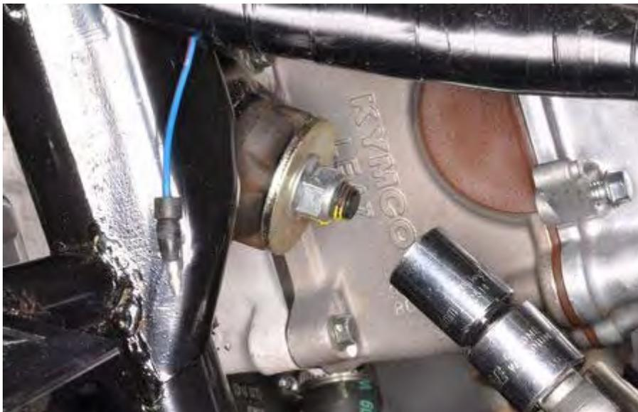
Tighten the damper nut securely with a 14 mm socket.
