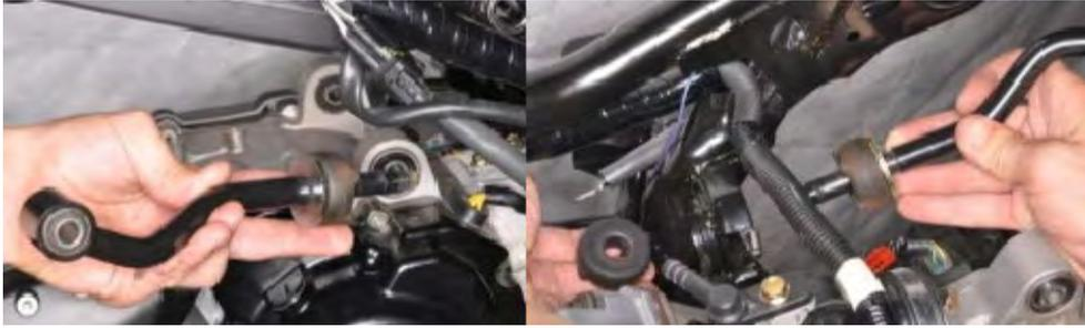
Fit the engine mounting bracket and damper assembly into place.
