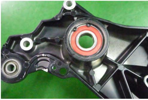
Install the snap ring into the groove.
