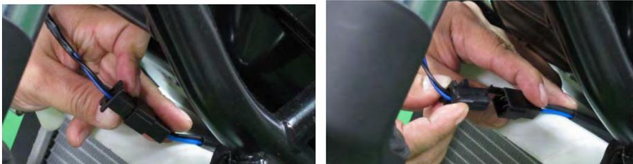
Unplug the cooling fan motor connector.
