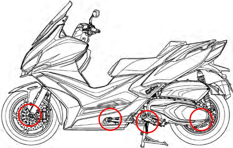
The frame lubrication points are listed below. Use general purpose grease. Apply clean engine oil or grease to cables and movable parts not specified. This will avoid abnormal noise and increase the durability of the motorcycle.
