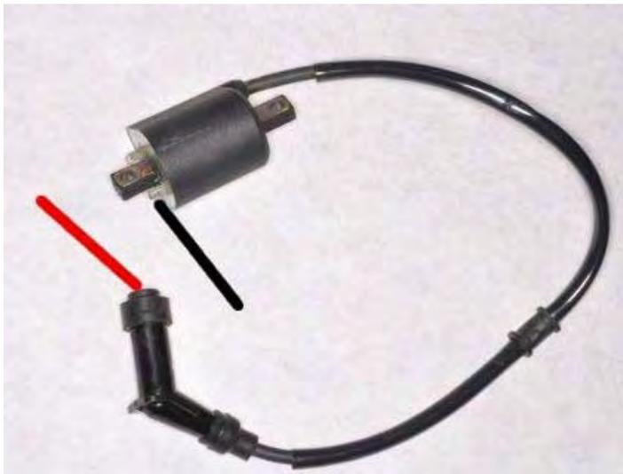
Check the secondary resistance between the ignition coil terminal and the spark plug cap. Touch the negative meter lead to the terminal and the positive meter lead to the spark plug cap as shown.
