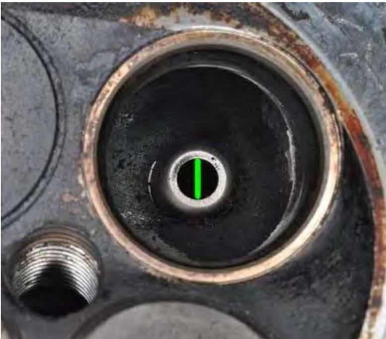
Measure the inside diameter of the valve guides. Replace the guides if the measurement is out of specification. Calculate the valve stem-to-guide clearance. Replace the guide and valve if the clearance is out of specification
