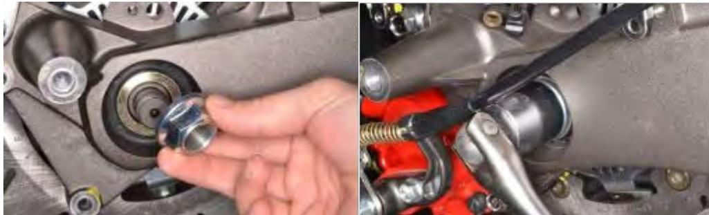
Install the rear axle nut and tighten it to specification with a 24 mm socket.
