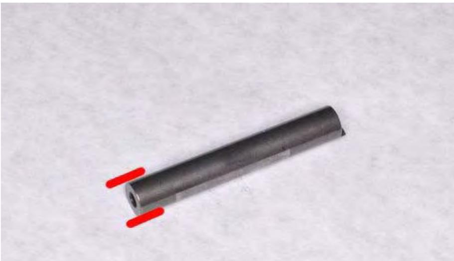
Inspect the rocker arm shaft outer diameter for the intake and exhaust valves.
