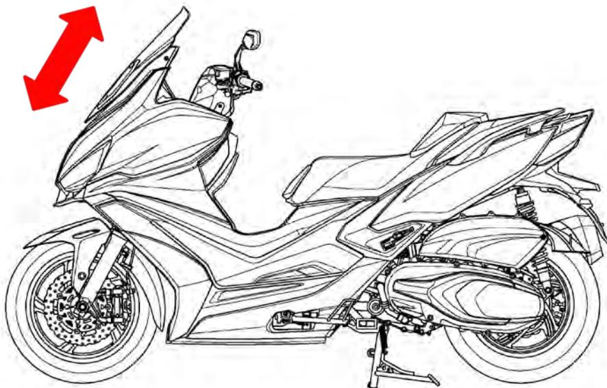
Check the action of the front shock absorbers by compressing them several times. Check the entire shock absorber assembly for oil leaks, looseness or damage.
