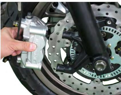
Remove the front brake caliper.
