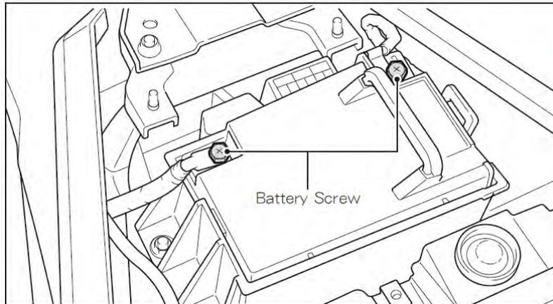
Check the battery voltage with a multi-meter. Place the positive probe onto the positive battery terminal and the negative probe to the negative battery terminal. If the battery reads under 12.3 V it is undercharged.
