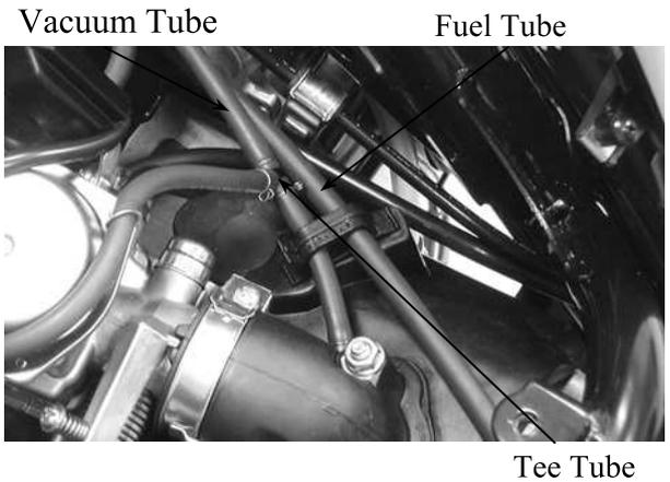
Disconnect the fuel tube at the carburetor side.
