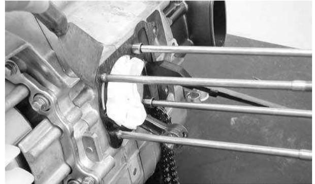
Install the piston, piston pin and a new piston pin clip.
