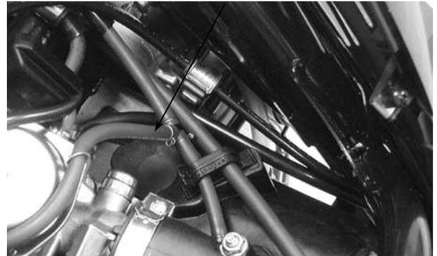
Connect the auto bystarter wire connector. Perform the following inspections and adjustments:
