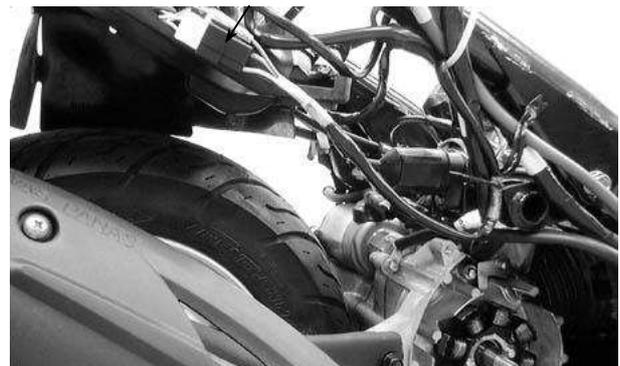
Remove the A.C. generator wire set plate.
