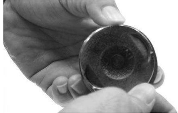
Install the piston rings onto the piston and measure the piston ring-to-groove clearance.
