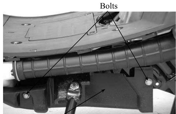
When installing, the edge of the bottom cover must be insert into the front side covers.
