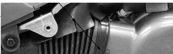
Install the drive belt air tube and tighten the
