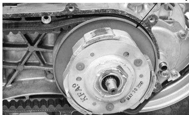
Hold the clutch/driven pulley assembly with
