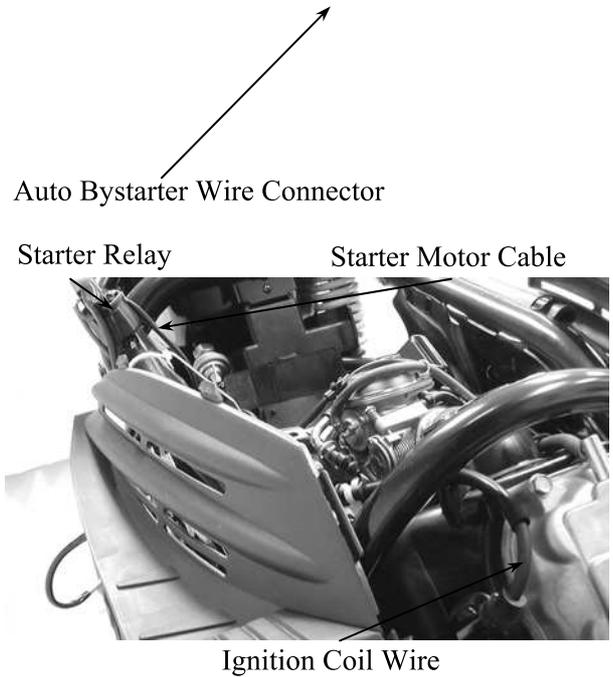
Disconnect the starter motor cable from the starter relay.
