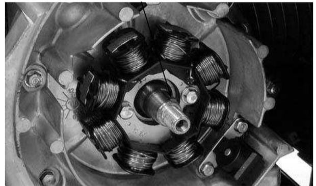
Install the flywheel onto the crankshaft with the flywheel hole aligned with the crankshaft woodruff key.
