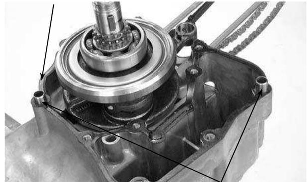
Remove the crankshaft and cam chain from the left crankcase.
