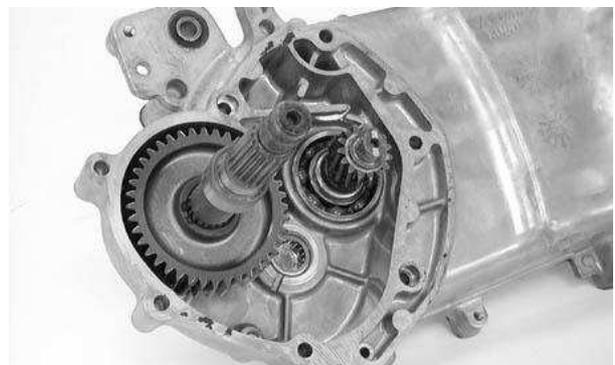
Install the countershaft and gear into the left crankcase.
