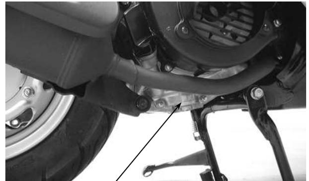
After the oil has been completely drained, check the filter screen O-ring for damage and replace if necessary. Install the oil filter screen, spring and filter screen cap.
