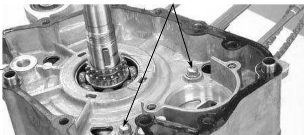
Remove the oil seal from the right crankcase.
