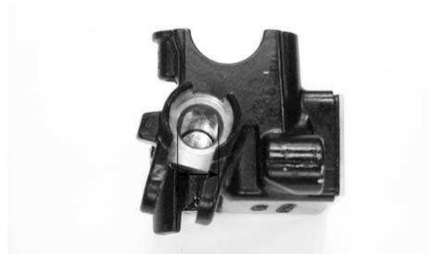
Measure the brake master cylinder piston O.D.
