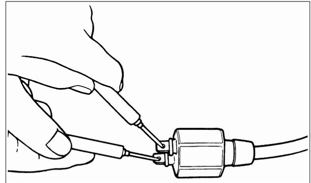
Measure the secondary coil resistances with and without the spark plug cap.
