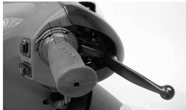
Major adjustment of the throttle grip free play is made at the carburetor side. Adjust by loosening the lock nut and turning the adjusting nut.
