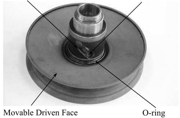
Remove the oil seal from the movable driven face.
