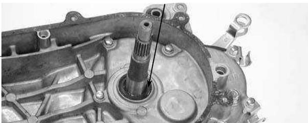
Check the left crankcase bearings for excessive play and inspect the oil seal for
