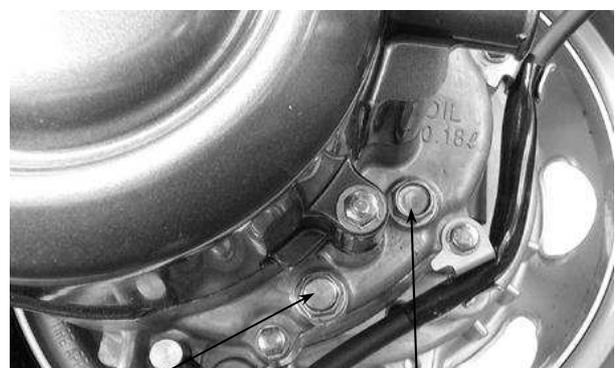
Drain Bolt Oil Check Bolt Hole/Oil Filler
