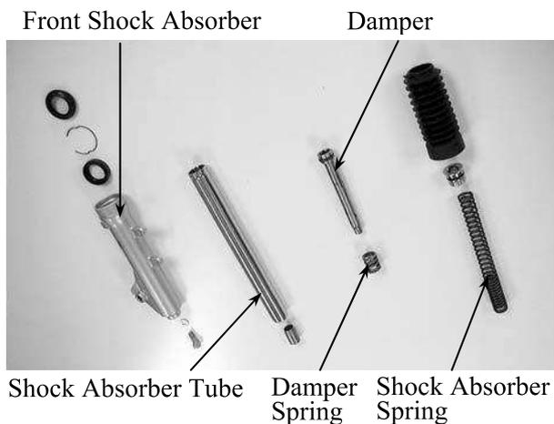
Shock Absorber Tube    Damper Spring    Shock Absorber Spring
