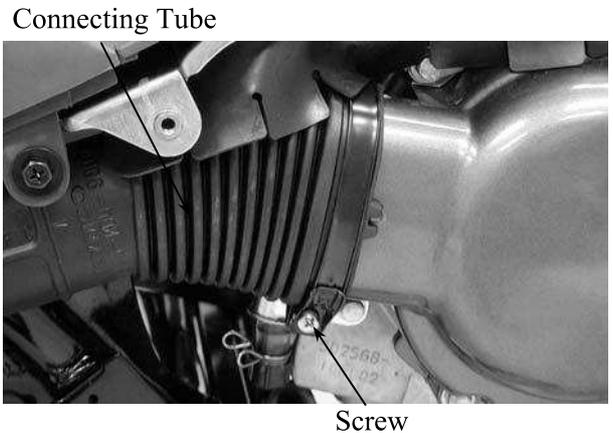
Loosen the drive belt air cleaner connecting tube band screw and remove the connecting tube.
