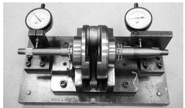
Turn the crankshaft bearings and check for excessive play.
