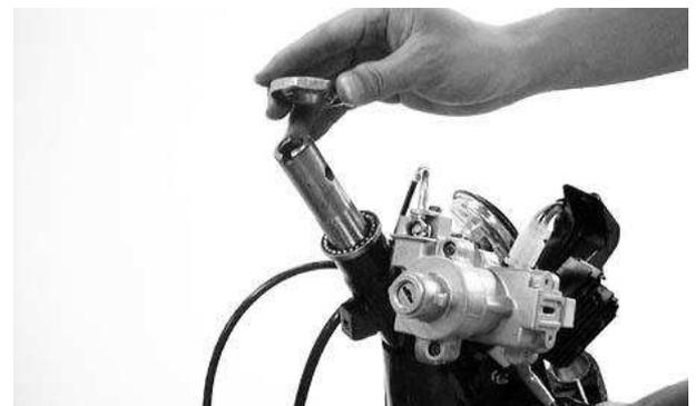
Apply grease to the top cone race and install
