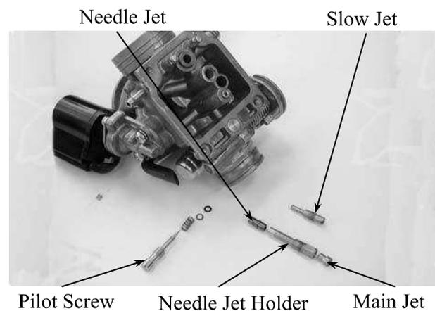
Clean the removed fuel jets with detergent oil and blow them open with compressed air.
