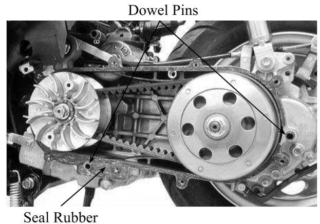
Install the left crankcase cover and tighten the left crankcase cover bolts.
