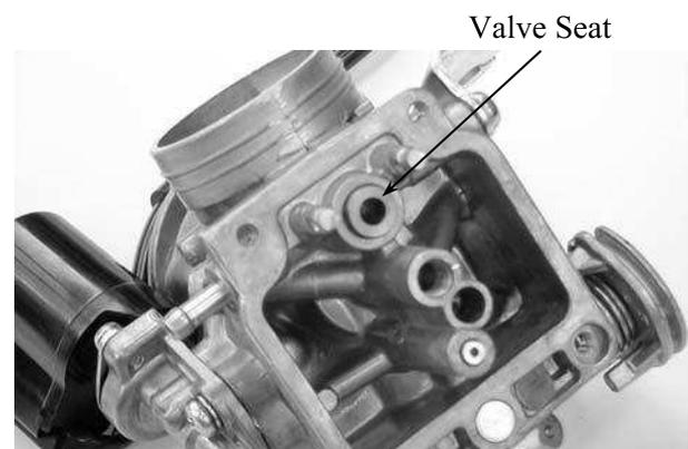
Remove the main jet, needle jet holder, needle jet, slow jet and pilot screw.
