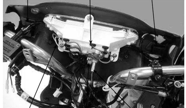
Fuel Gauge Wires Clamp Speedometer Cable
