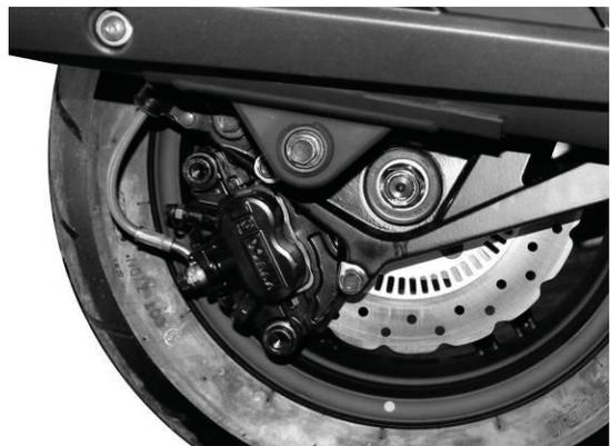
\* Keep grease or oil off the brake disk to avoid brake failure.
