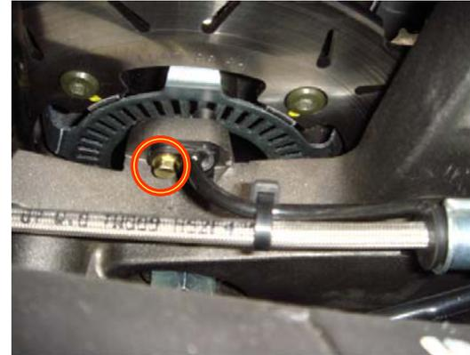
Remove the screw for rear wheel
