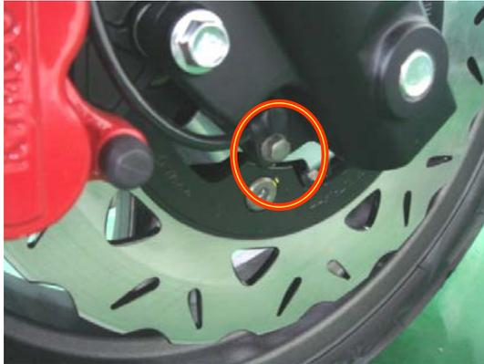
Remove the screw for front wheel
